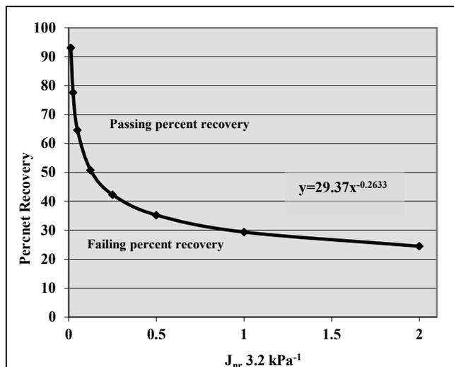
**Figure 4. Non-recoverable Creep Compliance versus Percent Recovery.**
