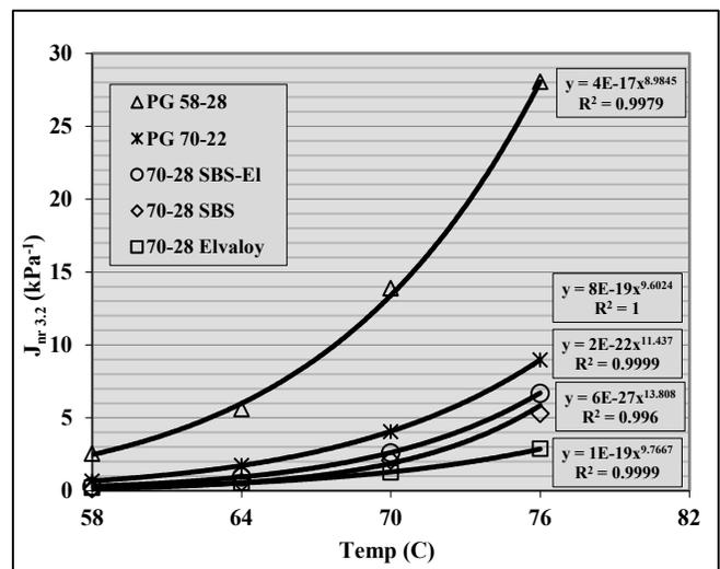
**Figure 6.  $J_{nr}$  3.2 Versus Temperature for Various AASHTO M 320 Graded PG 70 Binders.**
