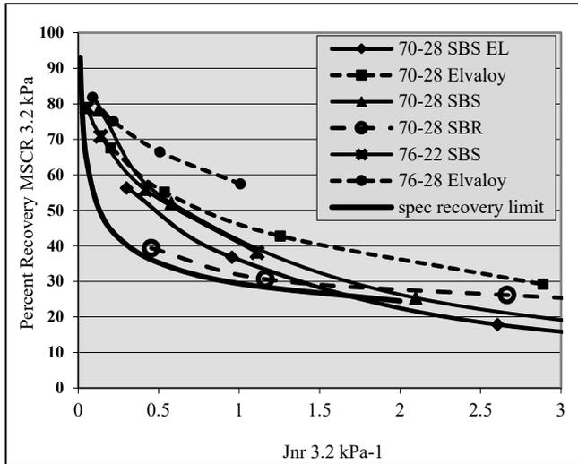
**Figure 5. MSCR Percent Recovery for Various Binders Modified with Elastic Polymers.**
