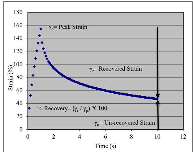
**Figure 1. MSCR Creep and Recovery Cycle.**
