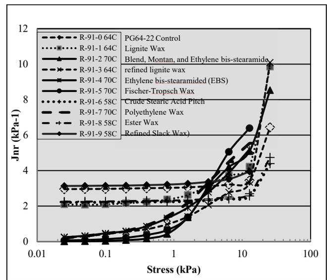
**Figure 3.  $J_{nr}$  versus Stress of Wax Modified Asphalt Binders.**
