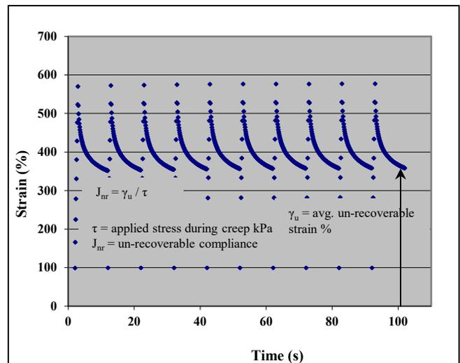
**Figure 2. Examples of Modified Asphalt Binder Response to Repeated Loading (D'Angelo et Al. 2007).**
