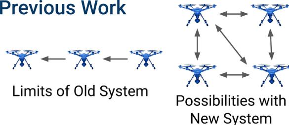
A previous system [2] enables drones to rely on another drone for positioning. Our work adds support for drones to rely on more than one drone, which means support for more swarm configurations. The arrows point from a drone to the drone that it relies on.
