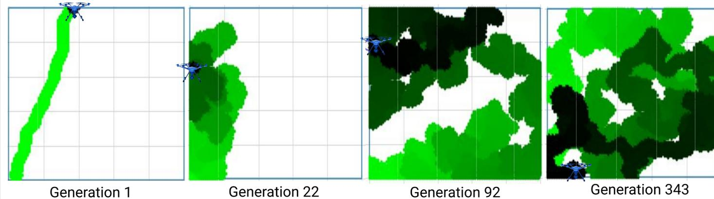
Shown above is one run of a simulated drone over many generations. The max area searched was 80.43%, which is typical for this algorithm. The drone is simulated for the same amount of time each generation, and survives if it covers more area than the previously fittest drone [3]. The lighter green represents earlier in the path, and the darker is later on. This correlates to the battery life of the drone over time.
