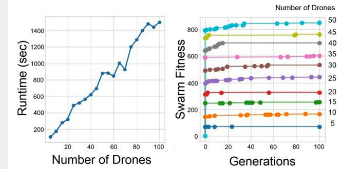
Left graph: The simulator was run for 300 generations with different numbers of drones. There is a linear correlation between runtime and number of drones.
