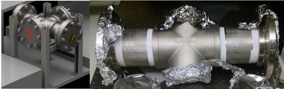
Fig. 3: Design (left) and flow-visualization experimental set up (right) for dropwise condensation
