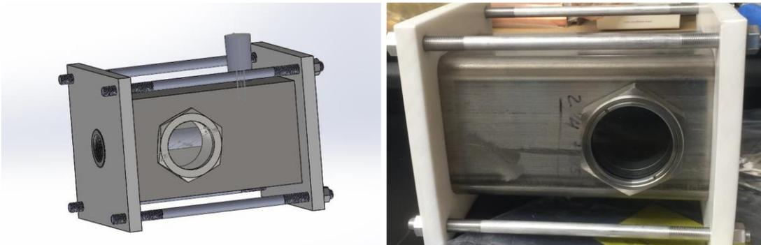
Figure 4: Design (left) and flow-visualization experiment (right) for pool boiling
