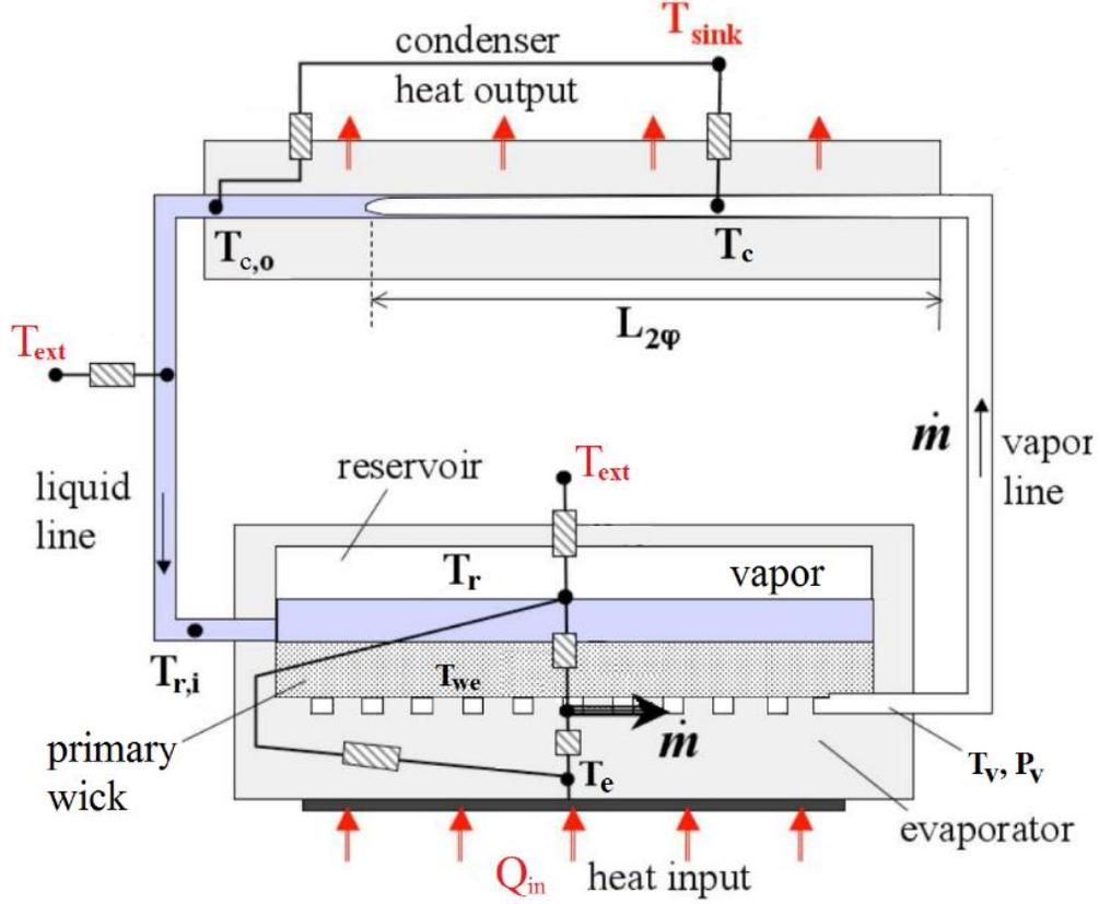
Fig. 1: Schematic of the LHP model [1] and its thermal resistance network [9].
