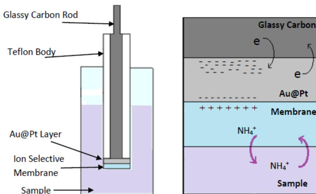
Figure 3-1: The scheme of the ion selective electrode (ISE) for ammonium detection as well as the illustration of the different layers of the ISE where Au@Pt nanoparticles are used as the solid contact.
