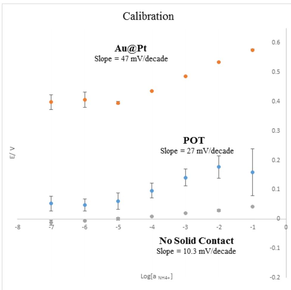
Figure 3-3: The calibration curves of the ISEs using Au@Pt nanoparticles, POT as solid contact, and the electrode without solid contact.
