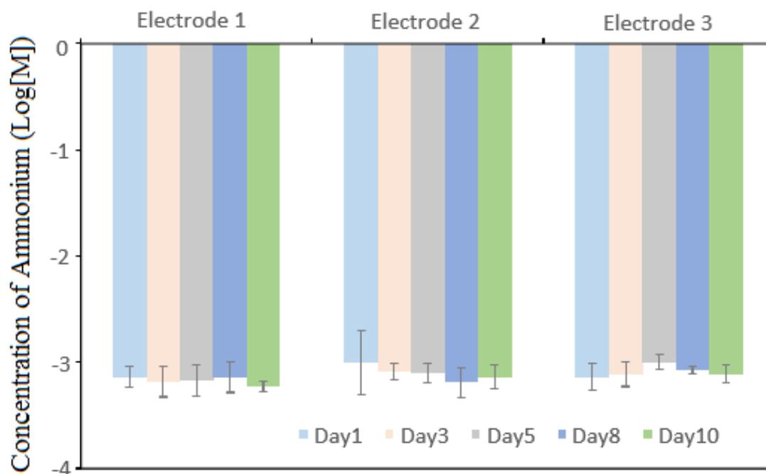
Figure 3-9: The measurement stability of three fabricated electrodes using the two-point calibration strategy for each measurement.
