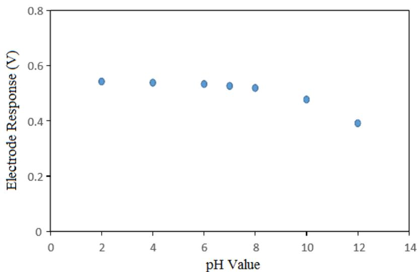
Figure 3-6: Effect of pH values on the response of the proposed electrode.
