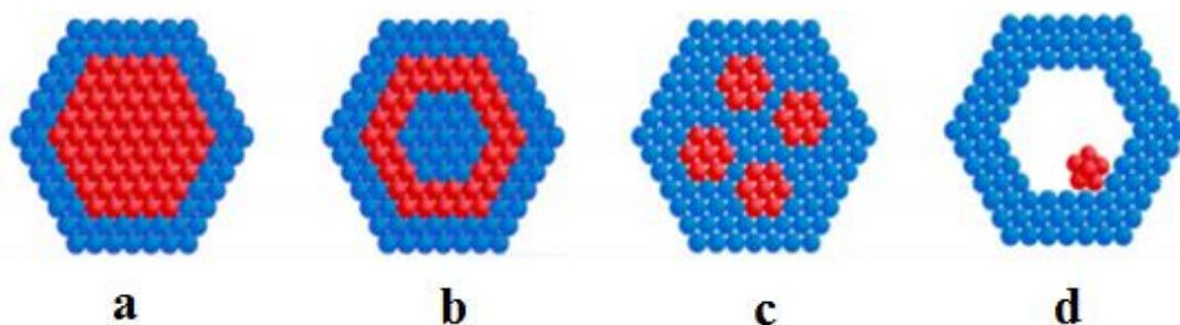
Figure 1-2: Structures of core-shell bimetallic nanoparticles: (a) Core-shell nanoparticles; (b) Multi-shell nanoparticles; (c) Multiple small core material coated by a single shell material, (d) Movable core within a hollow shell material [5-6].
