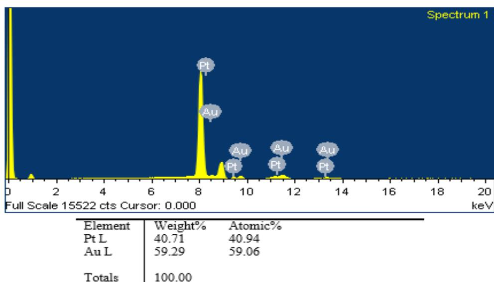
Figure 2-4: EDX results of Au@Pt particles and the percentage of each chemical in the Au@Pt nanoparticles.
