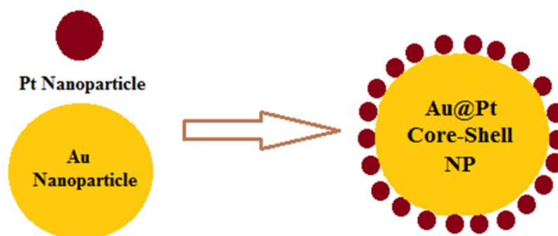
Figure 1-3: The general schematic of Au@Pt core-shell NP
