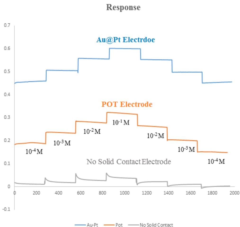
Figure 3-4: The electrode responses of the ISEs versus time with different ammonium concentrations for the three electrode configurations.
