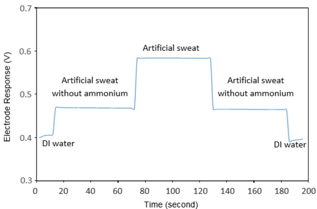
Figure 3-10: A representative real-world measurement of the artificial sweat using the proposed electrode. DI water and artificial sweat without ammonium were also measured as references.
