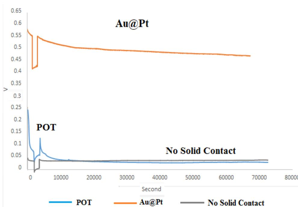
Figure 3-5: The water layer tests on the ISEs using Au@Pt nanoparticles and POT as solid contacts and the electrode with membrane only (no solid contact).
