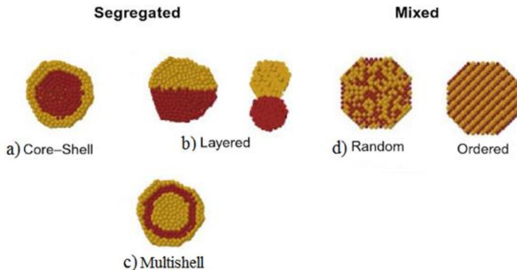
Figure 1-1: Types of chemical mixing patterns for nanoalloys [1-3].
