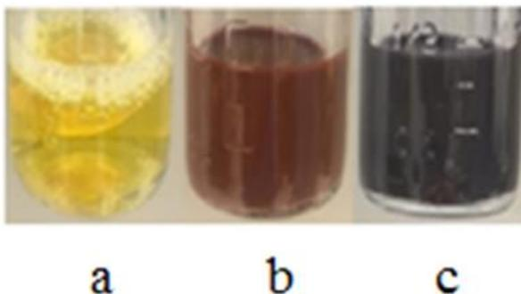
Figure 2-1: Au@Pt synthesis at different reaction times a) before adding ascorbic acid, b) after adding ascorbic acid and 15 minutes sonication, c) after 24 hours of stirring.
