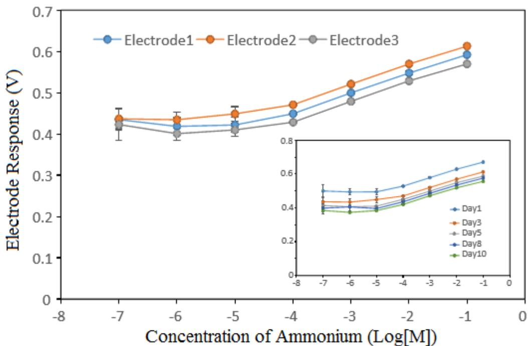
Figure 3-8: The repeatability testing results of three fabricated electrodes through measuring and comparing their calibration curves. The inset shows the drift of an individual electrode in the course of time.
