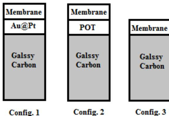
Figure 3-2: Three configurations of the ISE using different solid contact materials.
