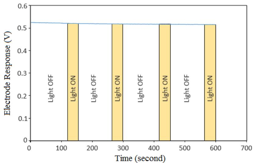
Figure 3-7: Effect of light on the response of the proposed electrode.
