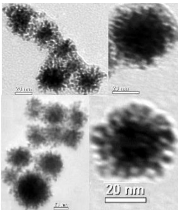
Figure 2-3: TEM images of Au@Pt core-shell NPs. (left) clusters of particles and (right) single particle.
