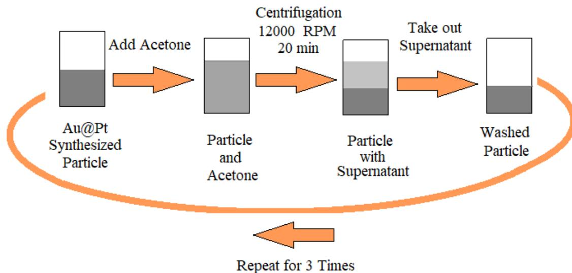
Figure 2-2: Washing procedure of the synthesized Au@Pt.
