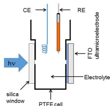
**Figure 2.** Schematic diagram of the experimental setup used in PEC current measurements.
