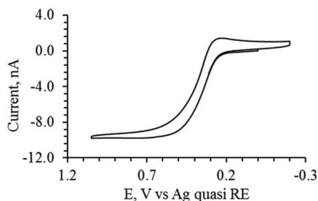
**Figure 4.** Cyclic voltammogram of a 40  $\mu\text{m}$  diameter disk in 0.78 mM ferrocene in MeOH with 0.15 M TBAP under an Ar atmosphere. The scan rate ( $v$ ) = 100  $\text{mV s}^{-1}$ .
