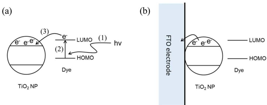
**Figure 1.** Schematics of the detection of DSNPs under illumination. a) Depicts light absorption and electron injection into the anchored NP by dye molecule. b) Describes the electron transfer from the DSNP interacting with FTO electrode.
