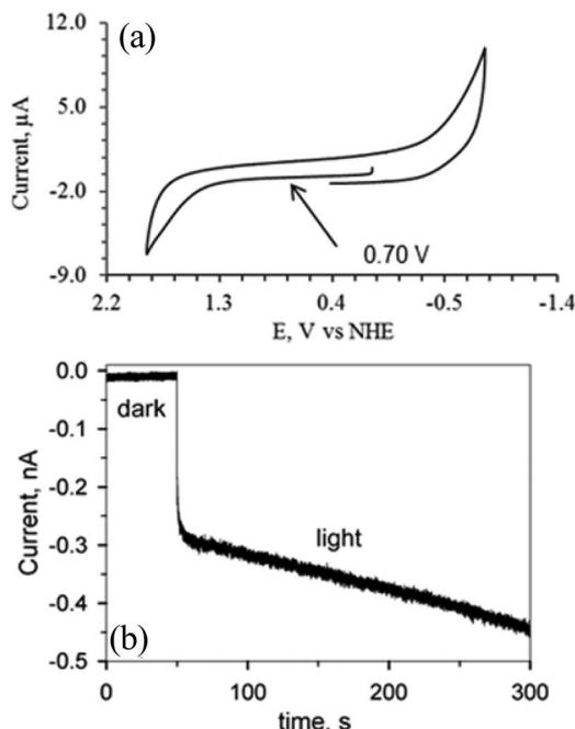
**Figure 5.** (a) Cyclic voltammogram of MeOH at FTO (diam = 0.7 cm) with 0.1 M TBABF<sub>4</sub>. (b) Background current for a 50  $\mu\text{m}$  diam UME at  $E_{\text{app}} = 0.7 \text{ V vs NHE}$ . The electrolyte was purified with activated alumina and purged with Ar for 20 min.
