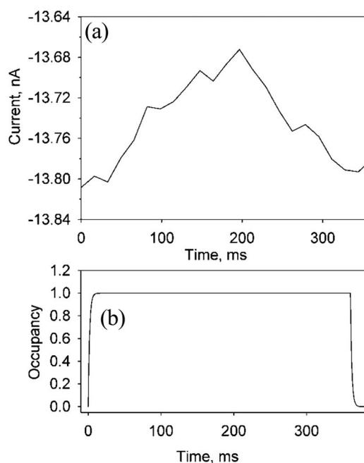
**Figure 13.** (a) Detail of a current transient and its comparison to the theoretical occupancy shown in (b) for a time constant,  $\tau = 12$  ms of the instrumentation.
