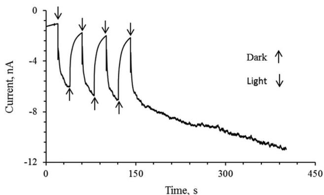
**Figure 7.** DSNPs suspension, 25 nM in MeOH with 0.1 M TBABF<sub>4</sub>, saturated with Ar. Data were collected by chopping light on ( $\downarrow$ ) and off ( $\uparrow$ ) in 20 s intervals during the initial 150 s.
