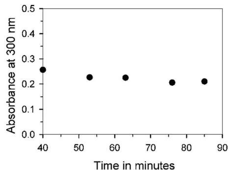
**Figure 8.** The absorbance vs time graph for 25 nM dye sensitized  $\text{TiO}_2$  NPs suspended in MeOH with 0.1 M TBAP. The absorbance was recorded at 300 nm. A quartz cell with 1 mm path length was used.
