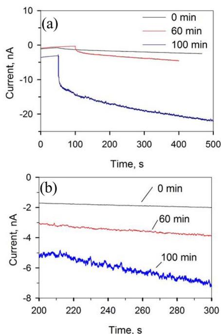
**Figure 9.** (a) Plot of current vs. time behavior for 25 nM DSNPs suspended in MeOH with 0.1 M TBAP. The data were collected over a period of time to study the effect of aggregations of NPs on PEC current transients. (b) Shows the data in (a) in detail.
