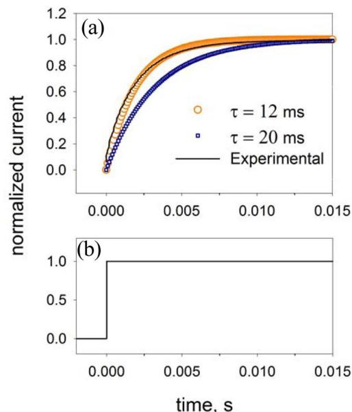
**Figure 12.** (a) Current transient from a potential step: (—) experimental results and the model applied to the transient, Eq. 4 with the best fit, (°, orange)  $\tau = 12$  ms and ( $\square$ , blue)  $\tau = 20$  ms. (b) Theoretical response or “occupancy” resulting from the step. For the experimental data in (a) the potential step was 0.05 V across  $R = 10$  M $\Omega$  with a final equilibrium current of 4.58 nA.
