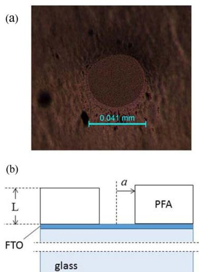
**Figure 3.** (a) Optical micrograph of FTO UME. (b) Schematics of the recessed disk.
