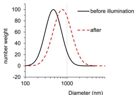
**Figure 11.** Dynamic light scattering data of a colloidal suspension of dye sensitized TiO<sub>2</sub> in MeOH, NP concentration of 25 nM in 0.1 M TBAP in MeOH. The data shows the size distribution before (—, black) and after (---, red) illumination for 20 min.
