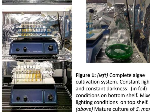
**Figure 1:** (left) Complete algae cultivation system. Constant lighting and constant darkness (in foil) conditions on bottom shelf. Mixed lighting conditions on top shelf. (above) Mature culture of *S. maxima*.
