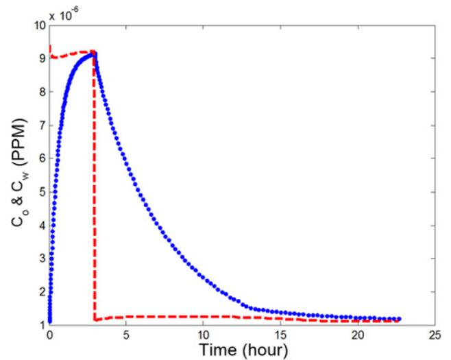
**Fig. 8**  $c_w$  and  $c_o$  as a function of time when a cooling happens at 3 h after a heating
