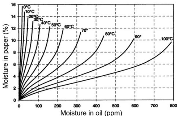
Fig. 1 MIT developed curves for water equilibrium in paper/oil system [19]
