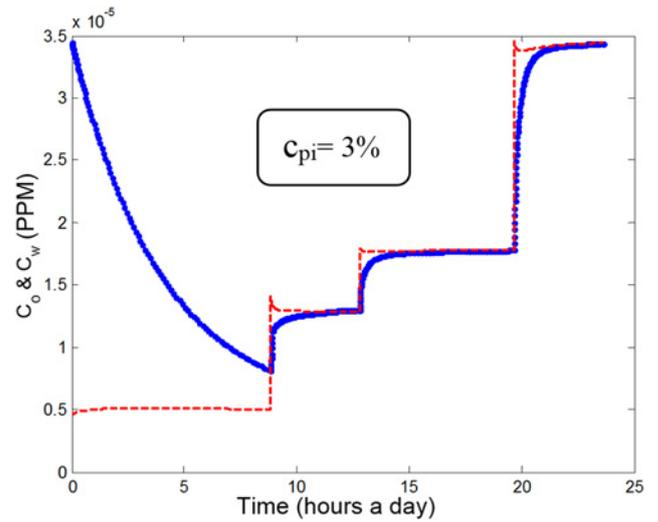
**Fig. 11** Concentration of water in the sublayer and oil as a function of time by using Table 2
