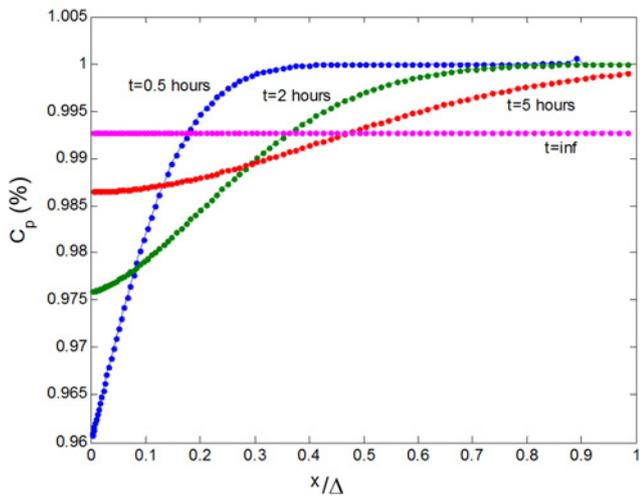
**Fig. 5** Spatial distribution of the concentration of water in the paper as a function of time when heating happens
