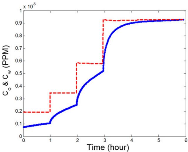
**Fig. 10**  $c_w$  and  $c_o$  as a function of time when a heating happens from 10 to 70°C during 4h
