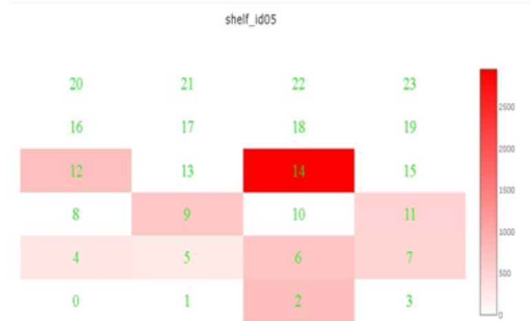
Figure 3.14: Example of isolation pattern. This figure shows that in a shelf with 24 devices, the majority of failure events occurred on an isolated device (14), while the neighboring devices (10,13,15,18) do not have any failure events.
