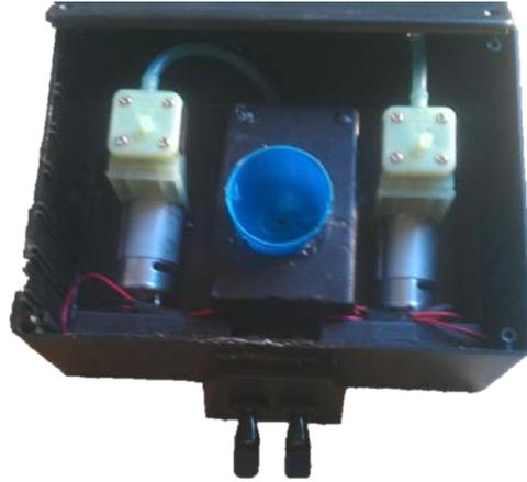
*Fig. 9. A picture of the vacuum compartment and the switch set-up in the lower box of phase two as seen in figure 4.*
