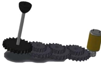
*Fig. 7. Isometric SolidWorks drawing of the gear system inside the bottom box in phase one. The far left gear is attached to the wheel and the far right gear is attached to the motor.*
