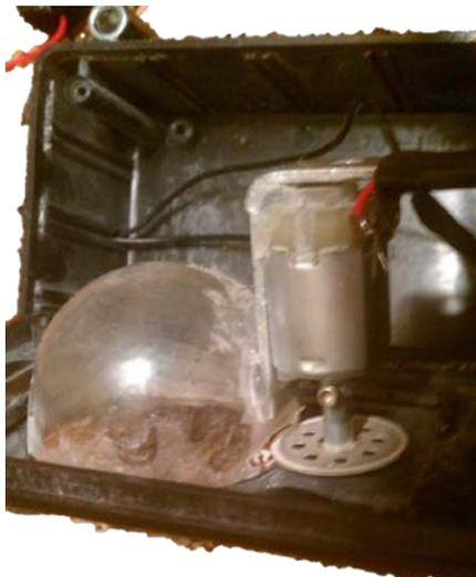
*Fig. 6. A view inside the upper box in phase one. This is a close-up of the blade-motor system and the plastic shell to hold the egg in place.*
