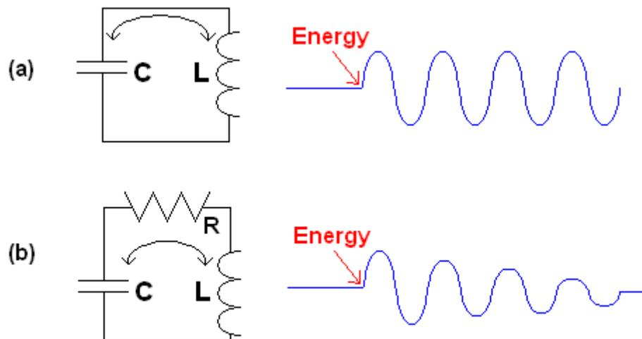
**Figure 3.3-1: Added Energy Initiates Sustaining Oscillations in an Ideal System (a) and Decaying Oscillations in a Lossy Practical Circuit (b).**
