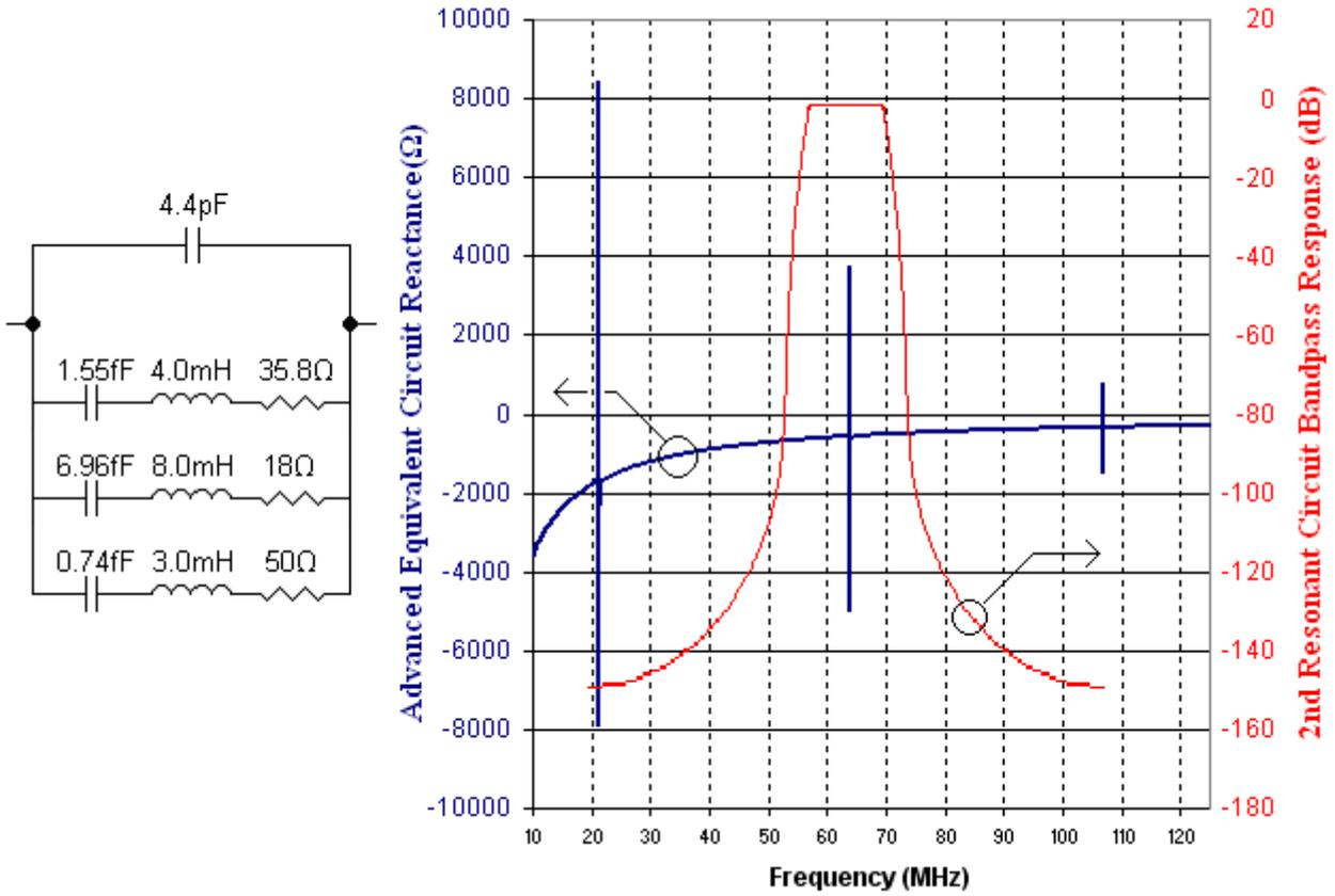
**Figure 4.2.3-1: 64 MHz Advanced Equivalent Circuit with Reactance Curve (blue) and 2<sup>nd</sup> Resonant Circuit Bandpass Response (red) Versus Frequency**
