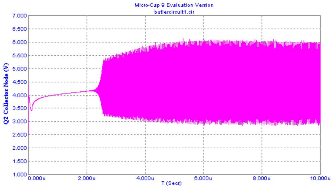
**Figure 5.2-1: Startup of Steady State Oscillations in Circuit Simulation**
