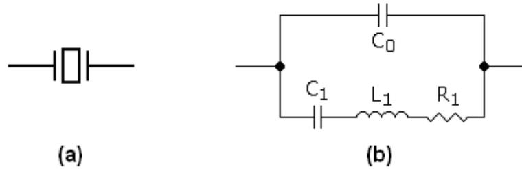
**Figure 4.2.1-1: Quartz Resonator Symbol (a) & Basic Equivalent Circuit (b)**
