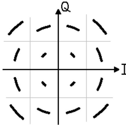
**Figure 2.1.1-2: Distortion of the 16-QAM by Frequency Synthesizer Phase Noise**
