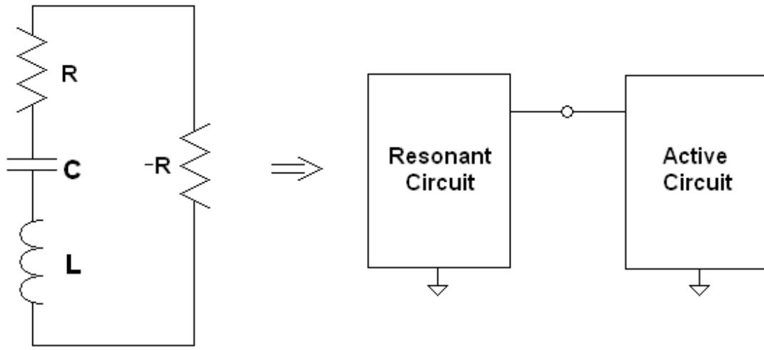
**Figure 3.4-1: Reconfiguration to One-Port Circuits**
