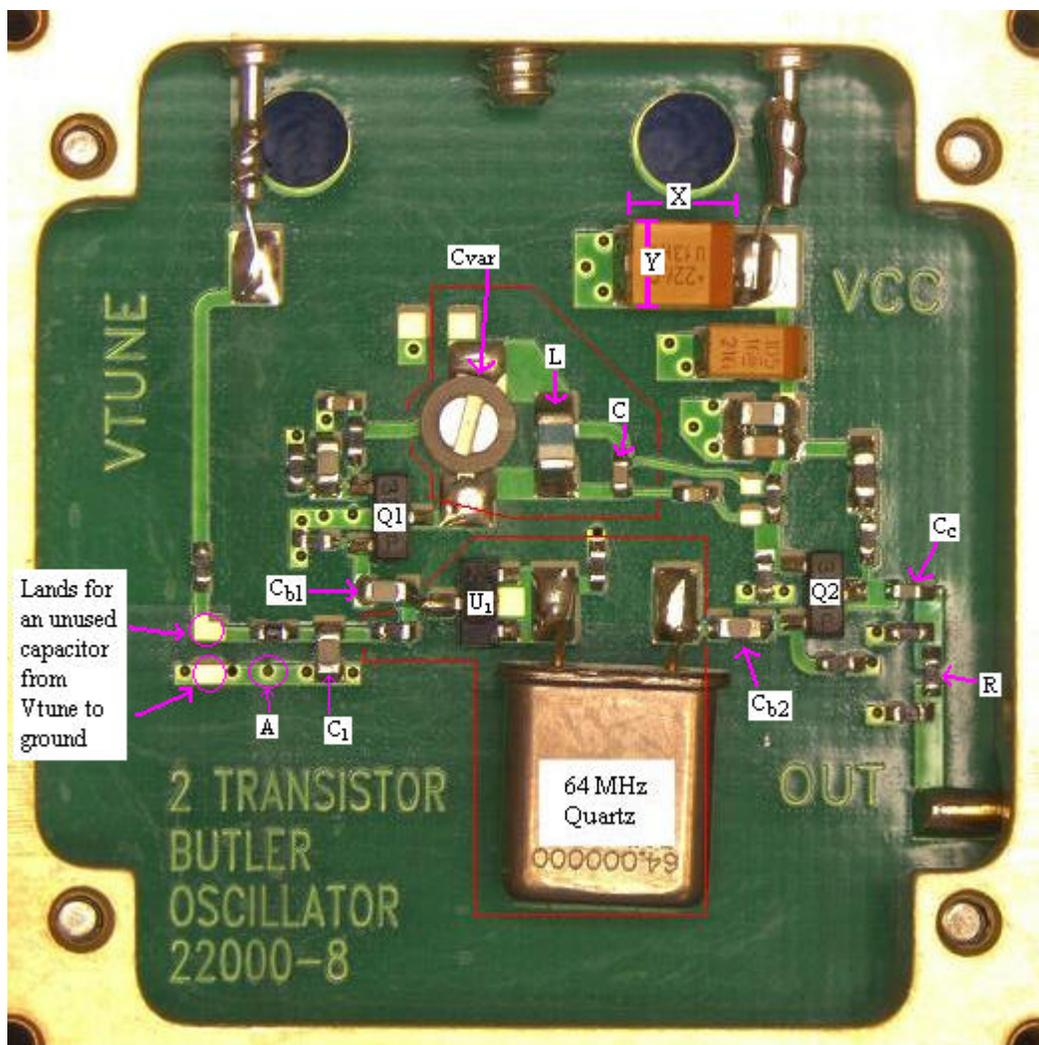
**Figure 5.3-1: Photograph of the Fabricated VCXO Circuit with Labels**
