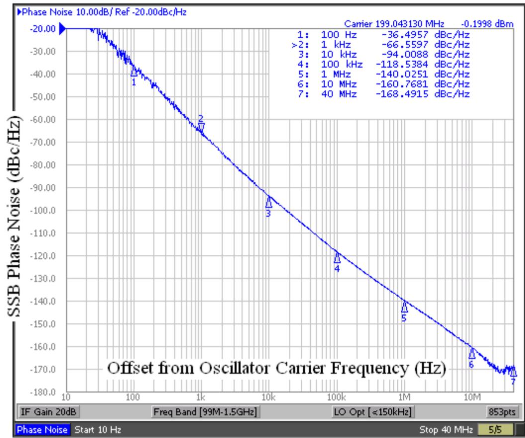
Figure 6.2-2: E5052A Phase Noise Measurement with 200 MHz Series RLC Resonator
