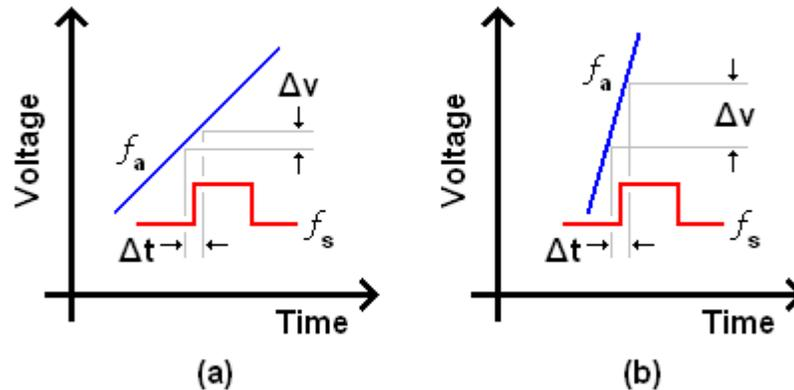
**Figure 2.3-2: Sampling Error in Low (a) and High (b) Frequency Analog Signals**
