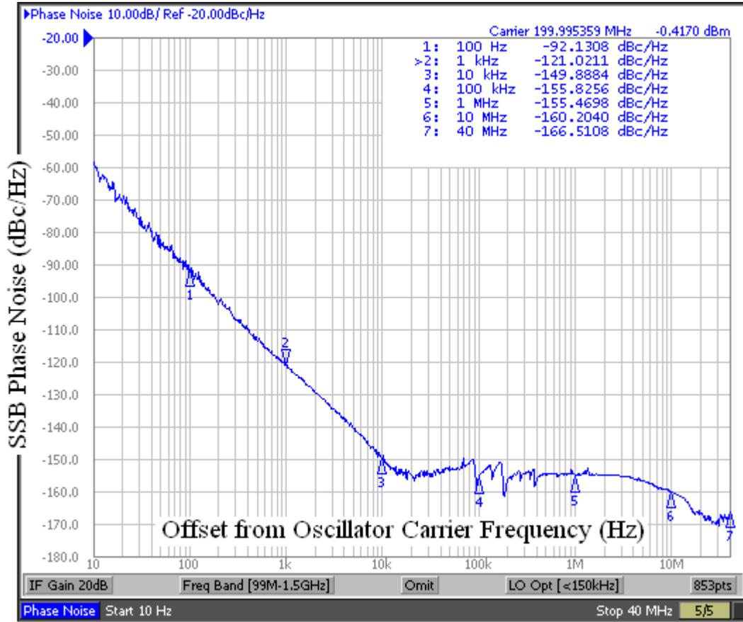
**Figure 7.3-2: E5052A Phase Noise Measurement with 200 MHz 3<sup>rd</sup> OT Inverted-Mesa Quartz Resonator**
