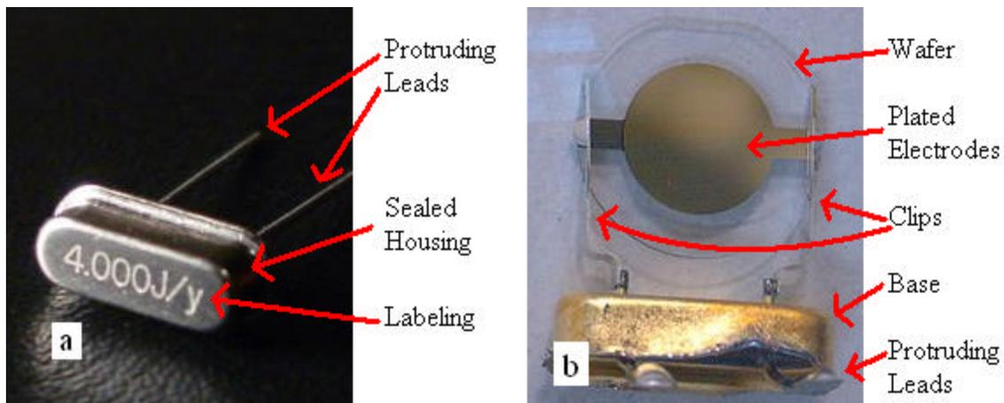
**Figure 4.1-2: Mounted Resonators with Cover In-Place (a) and Removed (b) [29]**
