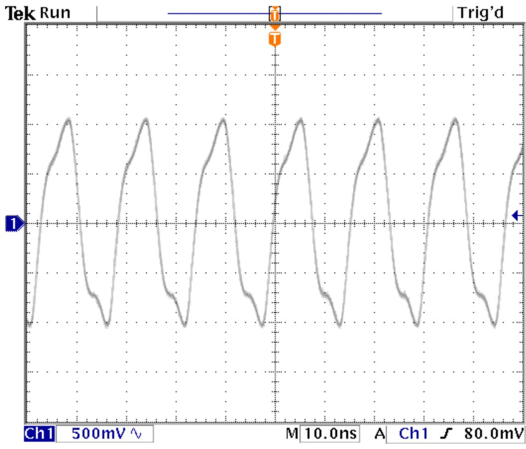
Figure 5.3-2: Measured Voltage Oscillation at Q2 Collector Node
