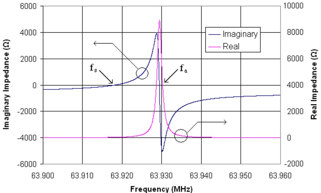
**Figure 4.2.2-2: Close-Up of Motional Arm Resonance**
