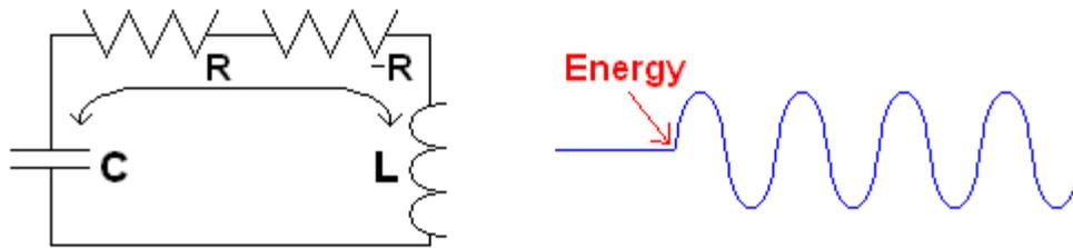
**Figure 3.3-2: Added Energy Initiates Sustaining Oscillations in Lossy Practical Circuit with Negative Resistance**
