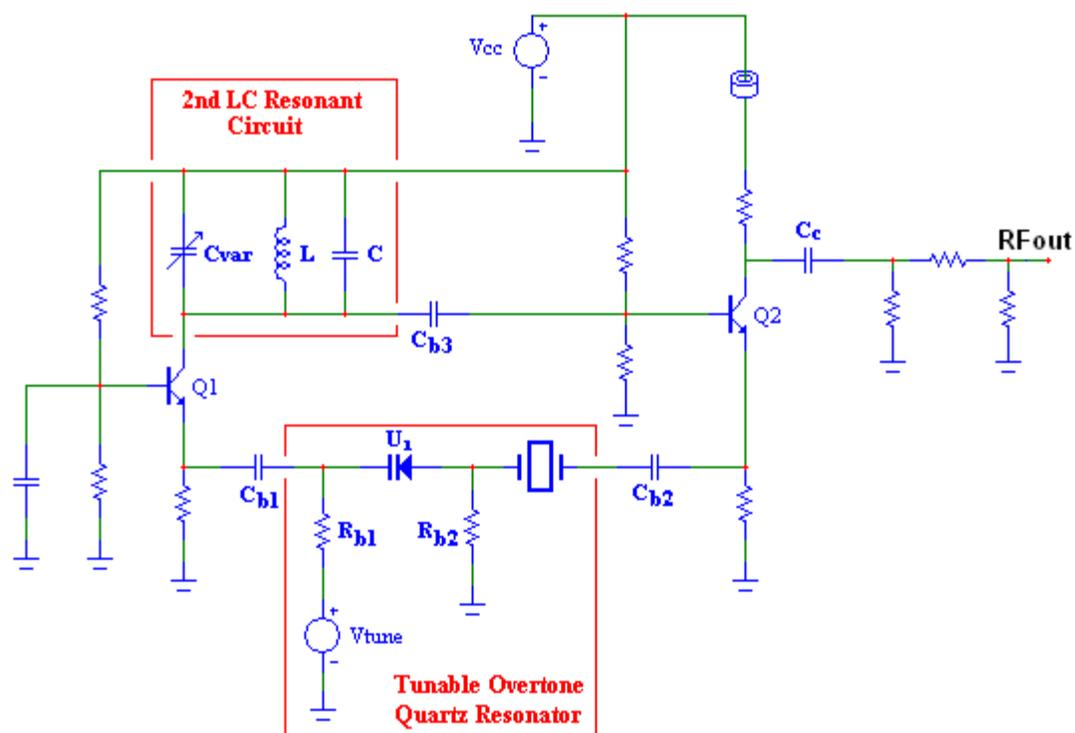
**Figure 5.1-2: Two-Transistor Butler Voltage Controlled Crystal Oscillator**
