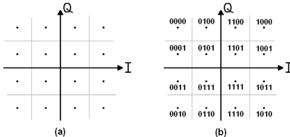
**Figure 2.1.1-1: (a) Ideal 16-QAM Showing Perfectly Modulated Data in Each Symbol. (b) Ideal 16-QAM with Grey Code Bit Assignment to Available Symbols.**
