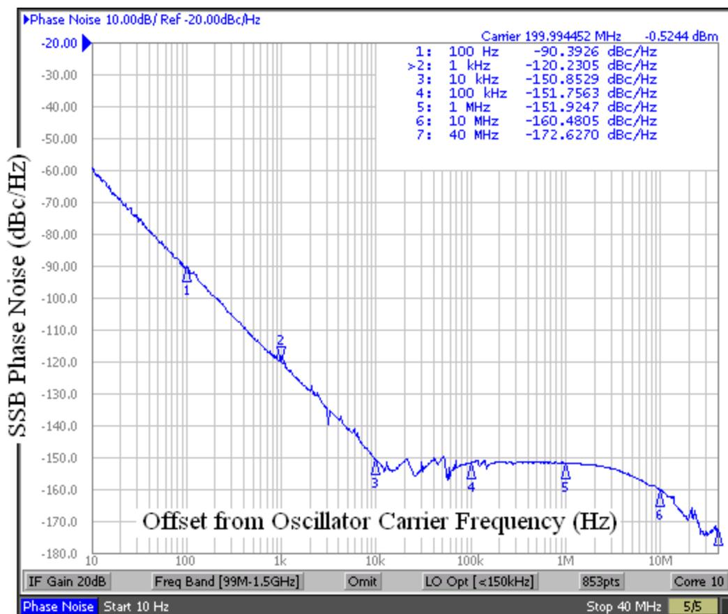
**Figure 6.3-2: E5052A Phase Noise Measurement with 200MHz 5<sup>th</sup> OT Quartz Resonator**
