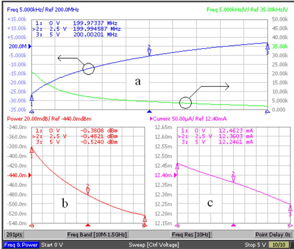
**Figure 6.3-1: Swept EFC Measurements with 200 MHz 5th OT Quartz Resonator. (a: blue) Oscillator Output Frequency. (a: green) Oscillator EFC Tuning Sensitivity. (b) Oscillator Output Power. (c) Oscillator Supply Current**
