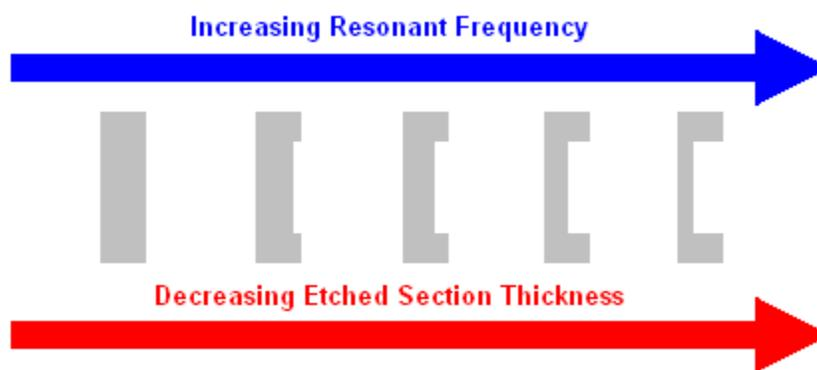
**Figure 4.3-1: Thickness vs. Resonant Frequency for Etched Resonator**
