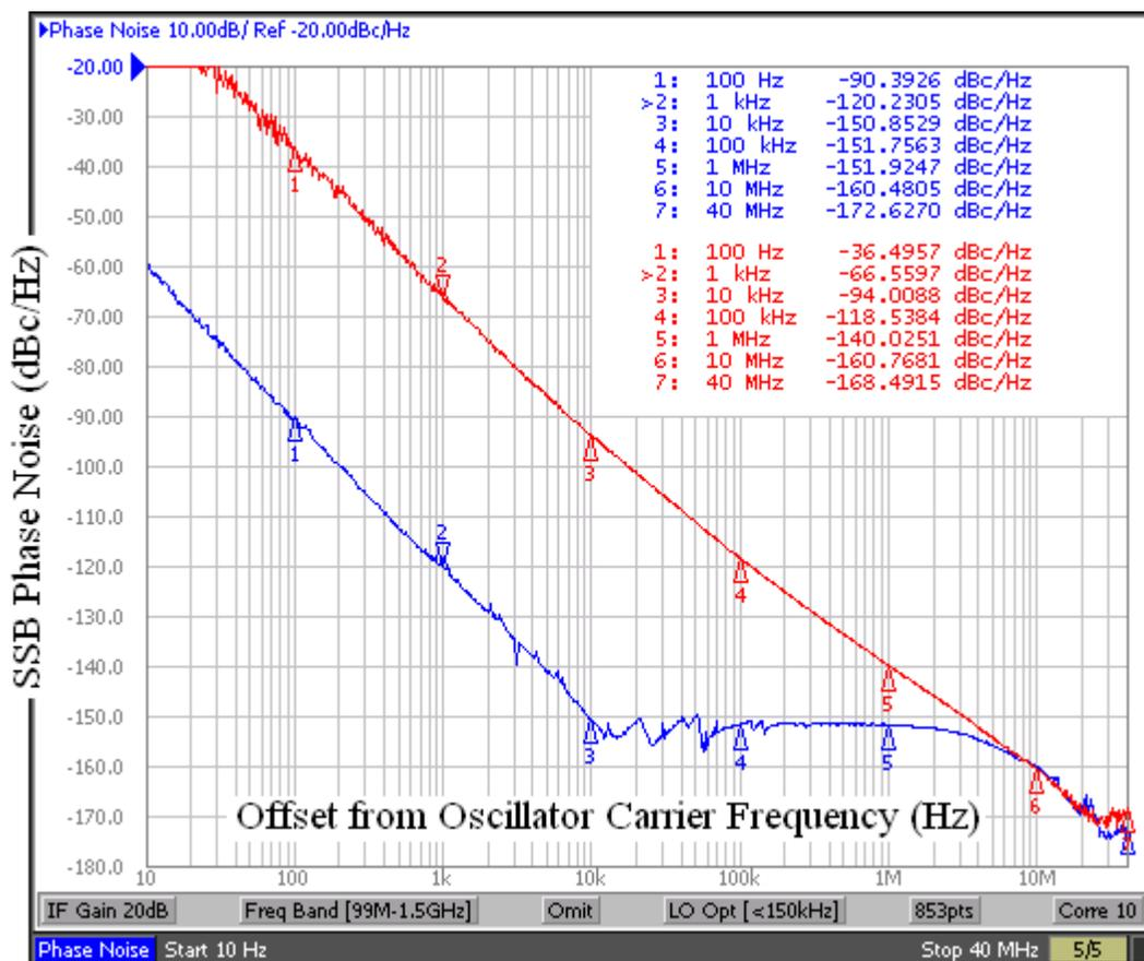
**Figure 6.4-1: E5052A Phase Noise Composite of 200 MHz Quartz and Series RLC Resonators**
