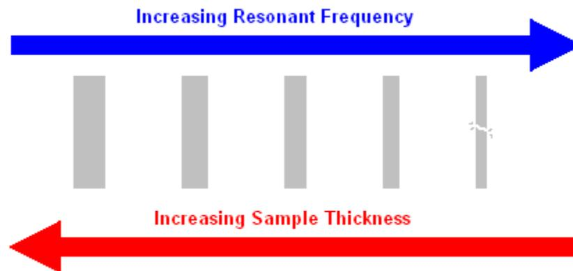
**Figure 4.2.4-1: Thickness vs. Resonant Frequency for Traditional Resonator**
