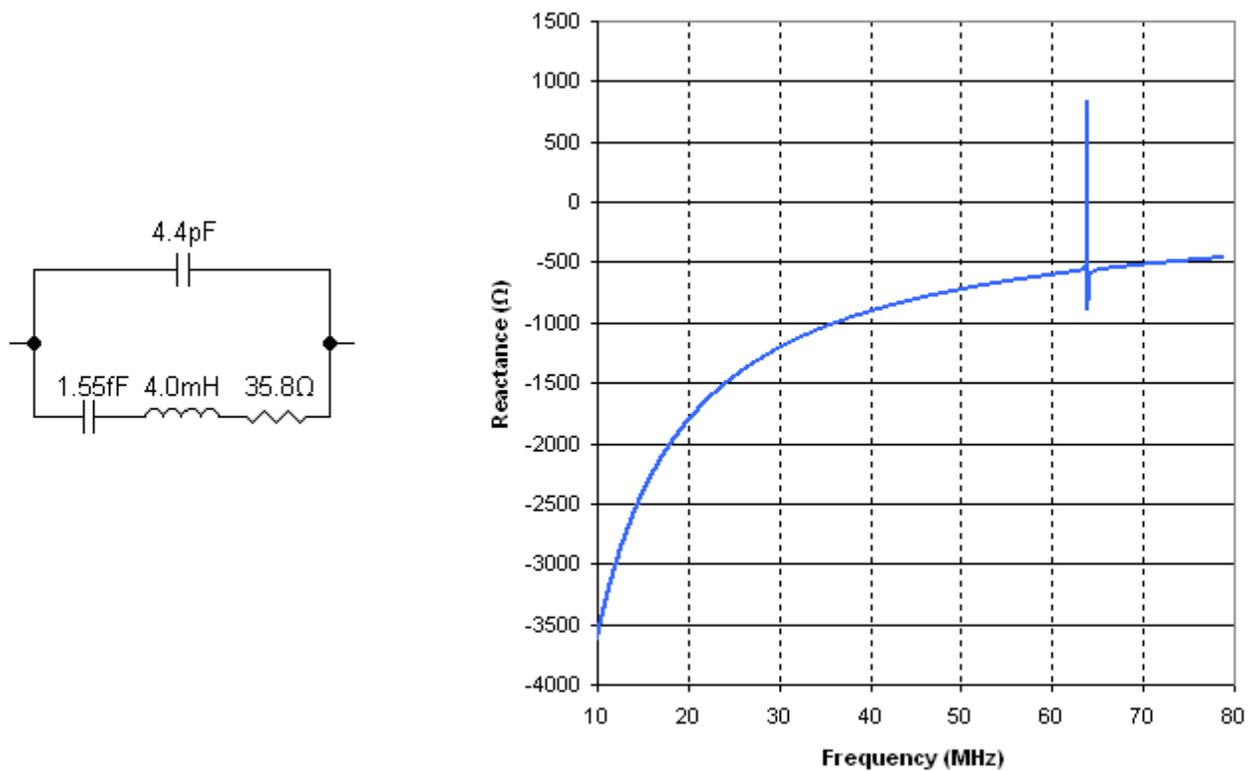
**Figure 4.2.2-1: 64 MHz Equivalent Circuit & Reactance Curve for the First 64 MHz Quartz Resonator in Table 4.2.2-1**
