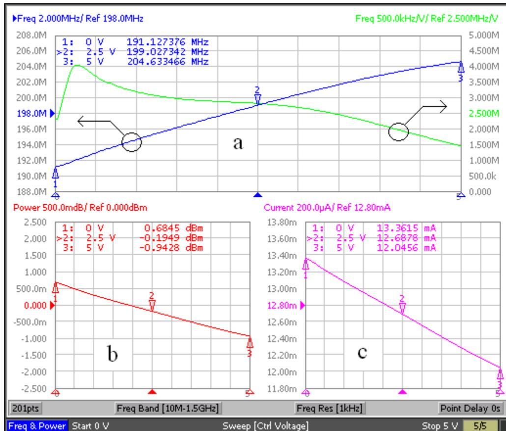
**Figure 6.2-1: Swept EFC Measurements with 200 MHz Discrete Series RLC Resonator. (a: blue) Oscillator Output Frequency. (a: green) Oscillator EFC Tuning Sensitivity. (b) Oscillator Output Power. (c) Oscillator Supply Current**
