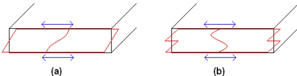
**Figure 4.1-1: Thickness Shear Mode Fundamental (a) and 3<sup>rd</sup> OT (b)**
