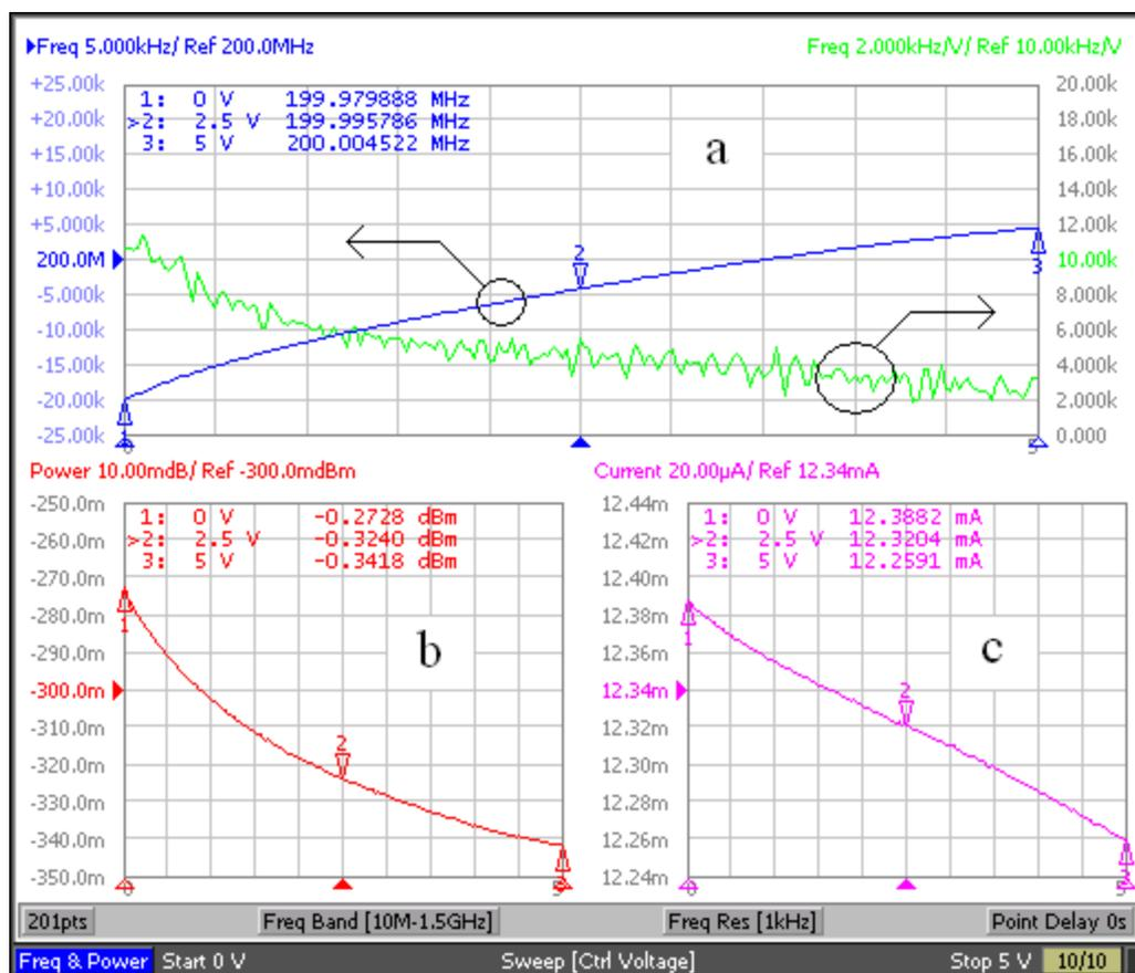
**Figure 7.3-1: Swept EFC Measurements with 200 MHz 3<sup>rd</sup> OT Inverted-Mesa Quartz Resonator. (a: blue) Oscillator Output Frequency. (a: green) Oscillator EFC Tuning Sensitivity. (b) Oscillator Output Power. (c) Oscillator Supply Current**
