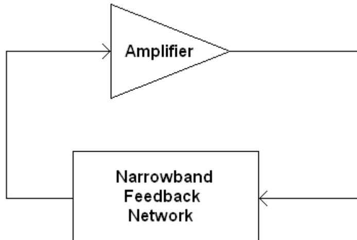
**Figure 3.2-1: Basic Oscillator Model**
