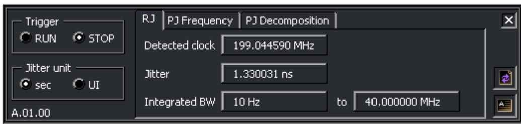
Figure 6.2-3: E5052A Time Jitter Integration with Series RLC Resonator
