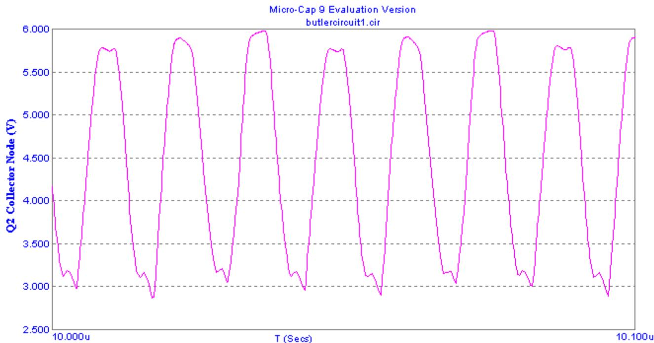
**Figure 5.2-2: Close-Up of Oscillations on Q2 Collector Node**
