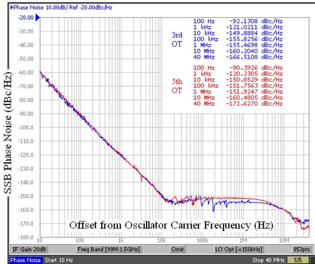
Figure 7.4-1: E5052A Phase Noise Composite of 200 MHz 5<sup>th</sup> OT Traditional and 3<sup>rd</sup> OT Inverted-Mesa Quartz Resonators
