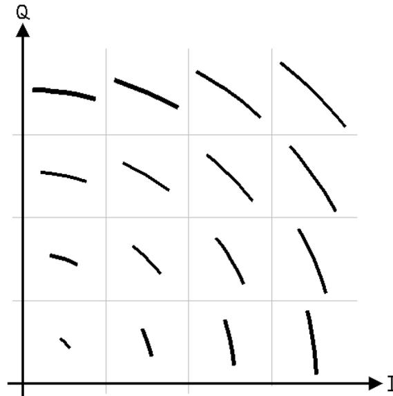
**Figure 2.1.1-3: 64-QAM with Phase Noise Distortion**
