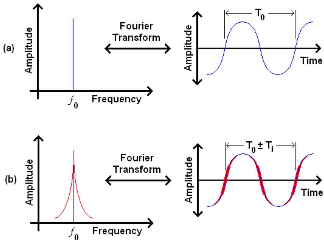
**Figure 2.3-1: Ideal (a) and Real (b) Oscillators in the Frequency and Time Domains**
