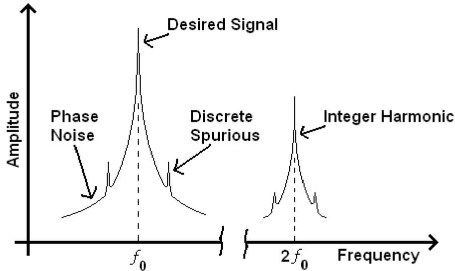
**Figure 1-1: Oscillator Output Showing Deteriorations in the Ideal Spectrum**
