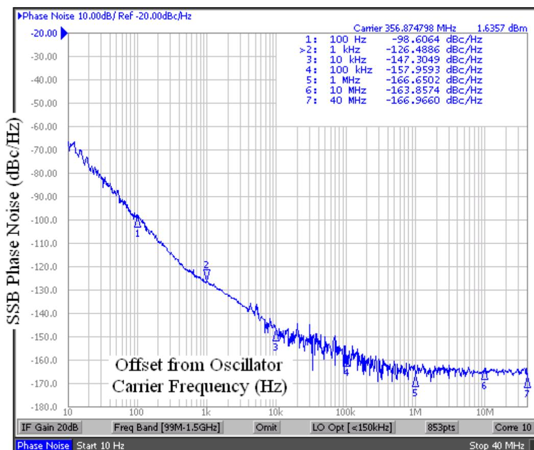
**Figure 8.2-2: E5052A Phase Noise Measurement of 356.875 MHz 3<sup>rd</sup> OT Inverted-Mesa Etched Quartz Resonator Based VCXO**
