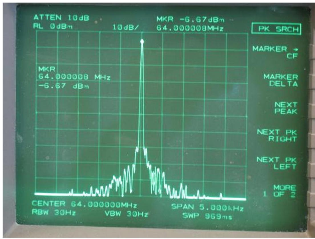
Figure 5.3-3: Spectrum Analyzer Display for Centered 64 MHz VCXO
