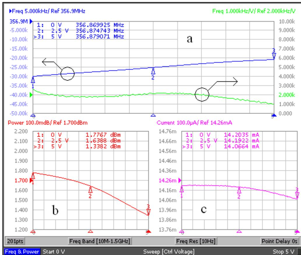
**Figure 8.2-1: Swept EFC Measurements with 356.875 MHz 3<sup>rd</sup> OT Inverted-Mesa Quartz Resonator. (a: blue) Oscillator Output Frequency. (a: green) Oscillator EFC Tuning Sensitivity. (b) Oscillator Output Power. (c) Oscillator Supply Current**
