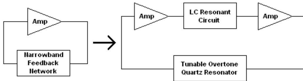
**Figure 5.1-1: Expansion of Most Basic Oscillator Model**
