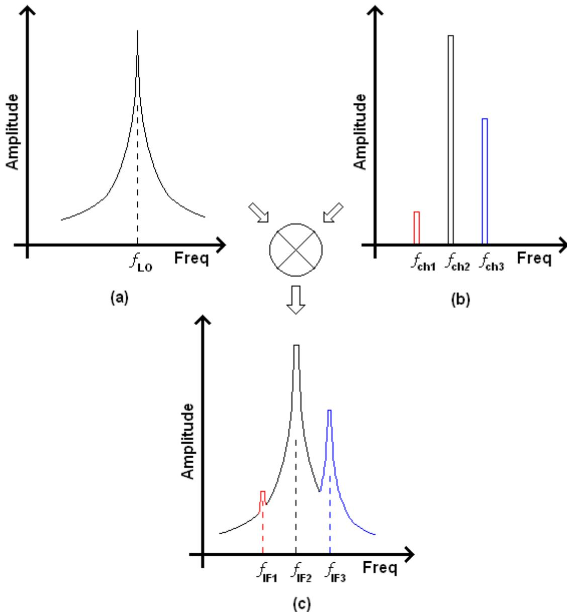
**Figure 2.1.2-1: (a) LO with Phase Noise. (b) Spectrum of RF Channels. (c) Selectivity Failure Due to LO Phase Noise Convolved with RF Spectrum.**
