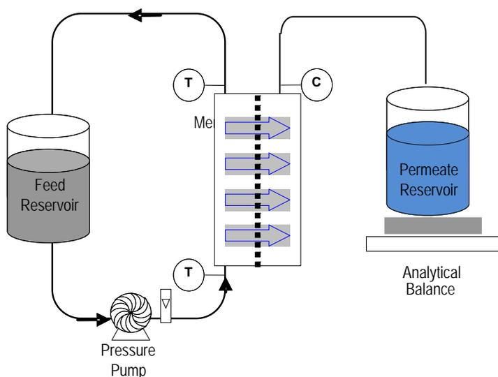
Figure 3. Schematic of NF and RO experimental system configuration.
