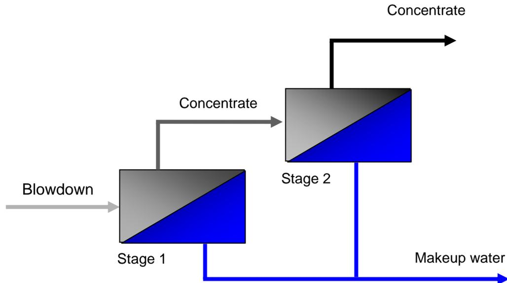
Figure 8. Schematic drawing of the modeled NF system. Stages have a variable number of pressure vessels and each pressure vessel has a variable number of membrane elements for the initial model. The second model has a constant number of pressure vessels and elements in each stage.
