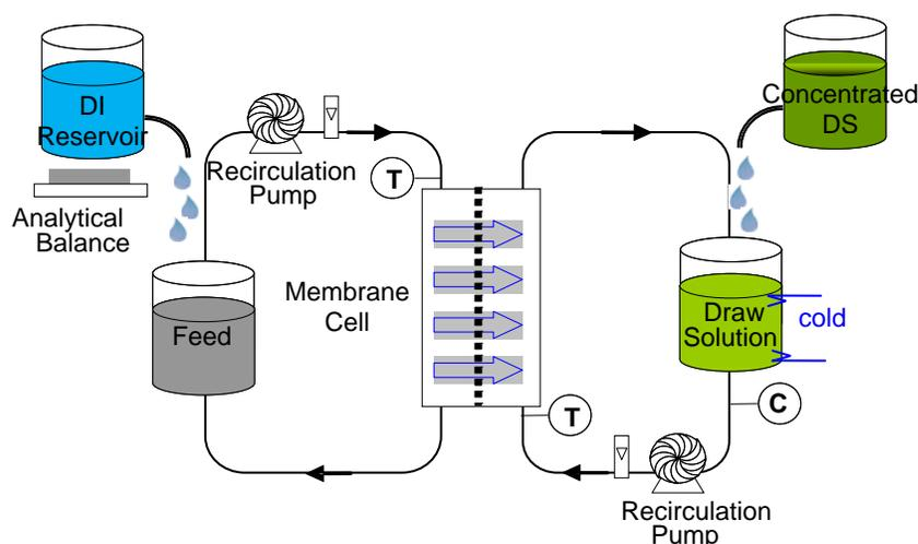
Figure 7. Schematic of bench-scale FO system.
