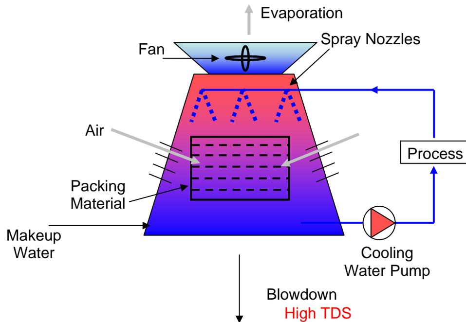
Figure 2. Flow diagram of recirculating, non-contact cooling loop with evaporative tower.
