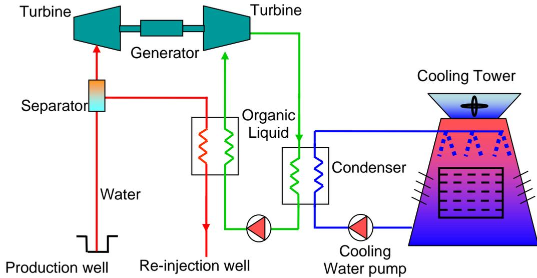
Figure 1. Schematic drawing of a combined flash steam-binary cycle geothermal facility. Electricity is produced in turbines by both super heated steam and organic vapors.
