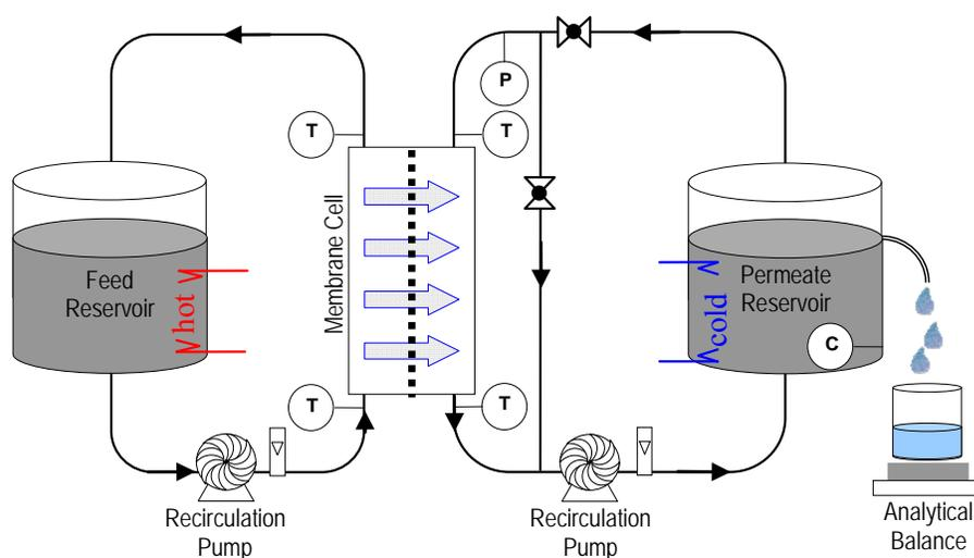
Figure 6. Schematic of bench-scale DCMD test system. Adapted from [29].
