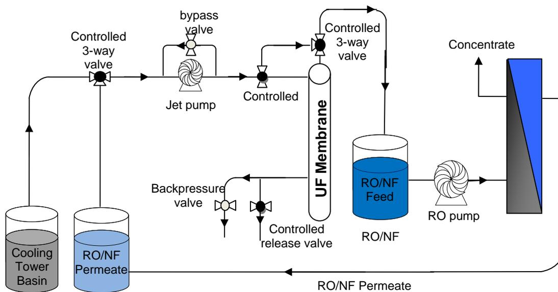
Figure 5. Schematic of flow of water through UF pretreatment system and the RO/NF pilot system.
