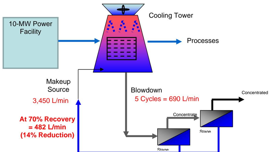
Figure 27. Schematic of cooling tower with the membrane system for treatment of blowdown brine. The permeate water is being reused as makeup water in the cooling tower.
