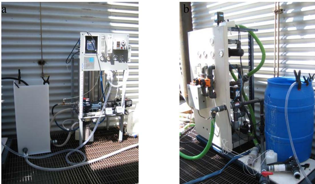
Figure 4. (a) RO/NF pilot system and (b) UF pretreatment system.
