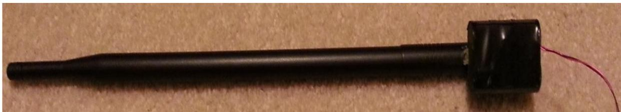
**Figure 17:** Final Prototype 2.0 Dipole Antenna
