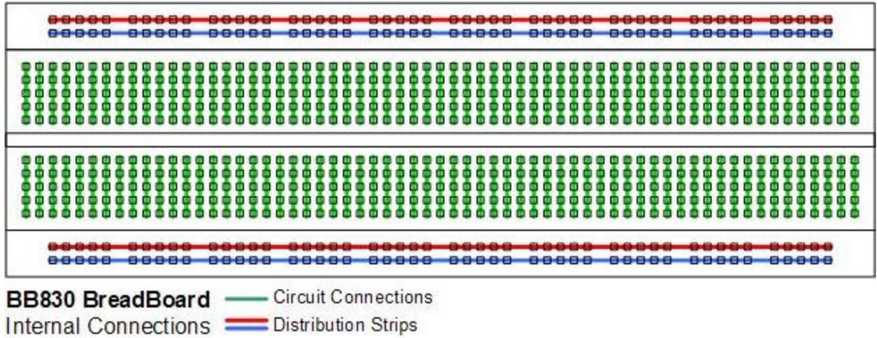
**Figure 13:** Internal Breadboard Schematic (BusBoard)
