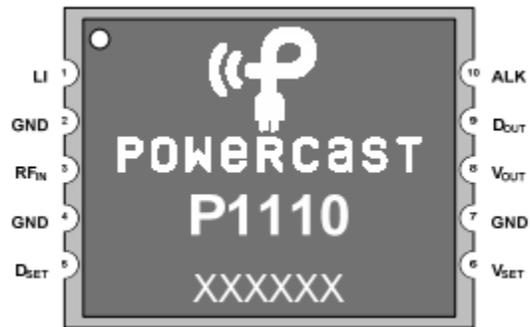
Figure 5: P1110 Pin Configuration (Wireless)
