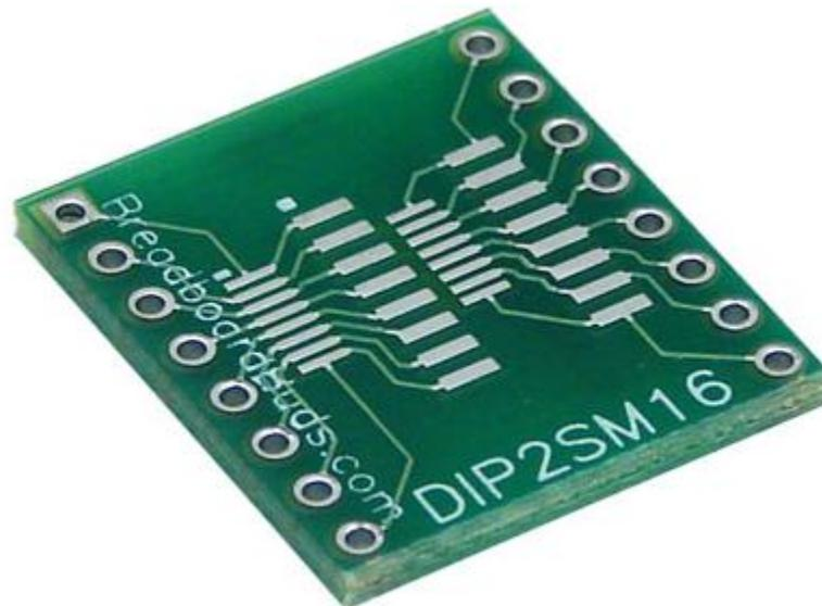
**Figure 14:** PCB Carrier (Technologicalarts)
