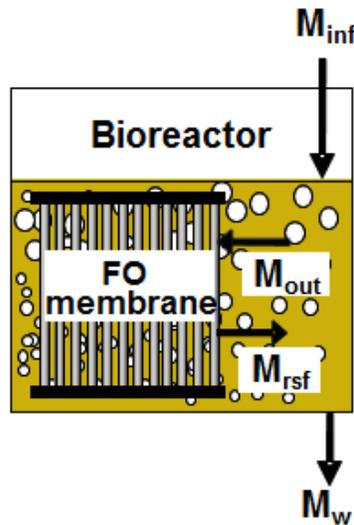
Figure 2. Schematic of an OMBR process salt mass balance.
