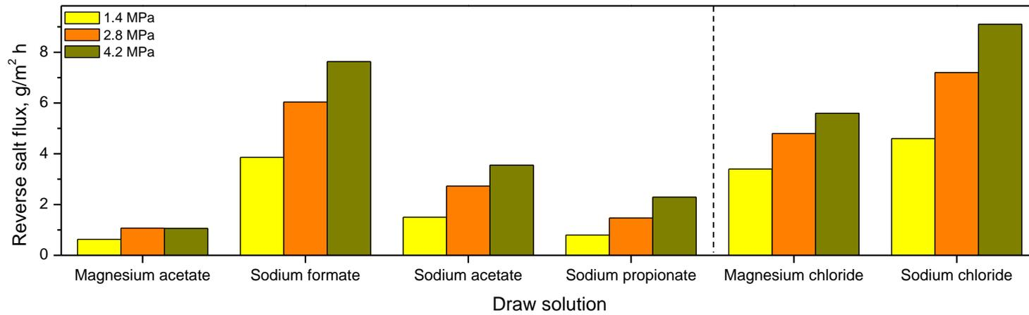
Figure 8. Comparison of reverse salt diffusion ( $J_s/J_w$ ) for all the organic salts at each osmotic pressure tested with sodium chloride and magnesium chloride results from Ref. [5].
