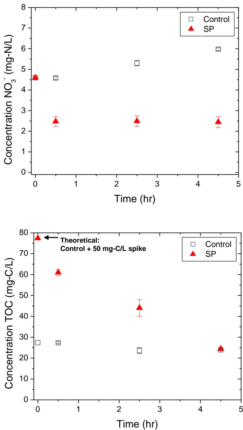
Figure 10. Concentration of a)  $\text{NO}_3^-$ -N and b) TOC as a function of time in an aerobic environment batch experiment, Samples taken from a membrane bioreactor and spiked with 133 mg/L of sodium propionate (SP), equivalent to 50 mg-C/L, are compared to membrane bioreactor control samples.
