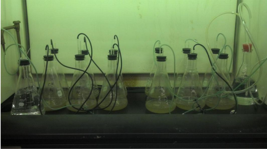
Figure 7. Batch experiment setup to determine effects of draw solute on biological performance. Six flasks were bubbled with  $\text{N}_2$  to simulate anoxic conditions (left), and six flasks were bubbled with air to simulate aerobic conditions (right).
