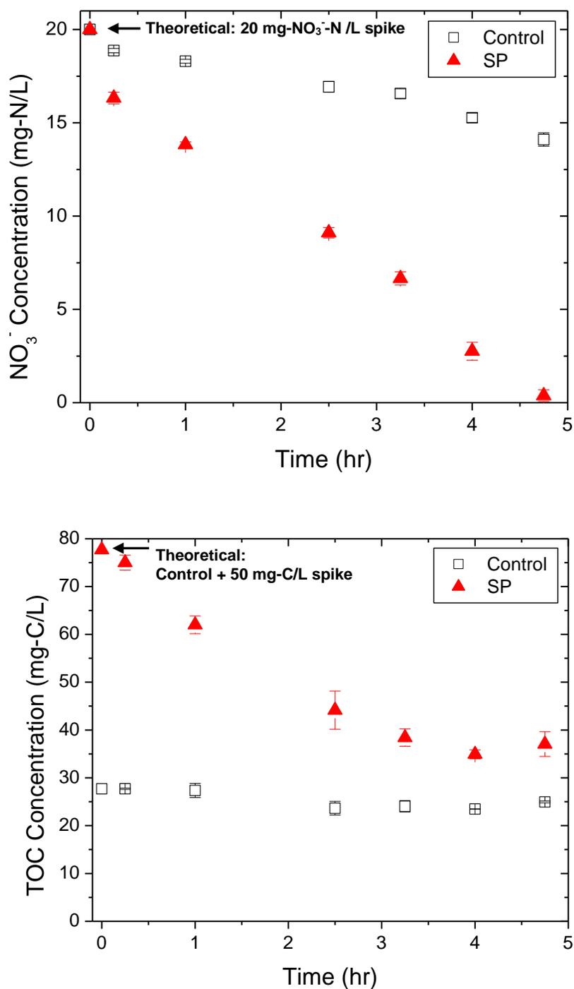
Figure 9. Concentration of a)  $\text{NO}_3^-$ -N and b) TOC as a function of time in an anoxic environment batch experiment. Samples were taken from a membrane bioreactor and spiked with 133 mg/L of sodium propionate (SP), equivalent to 50 mg-C/L, are compared to membrane bioreactor control samples.
