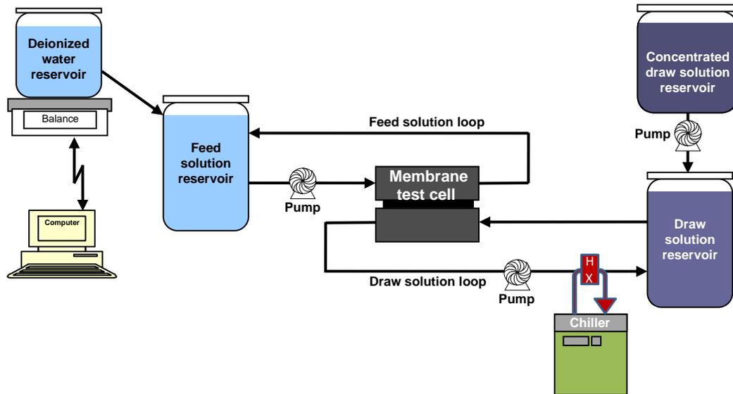
Figure 4. Schematic of bench-scale FO system. Figure adapted from Ref. [5].
