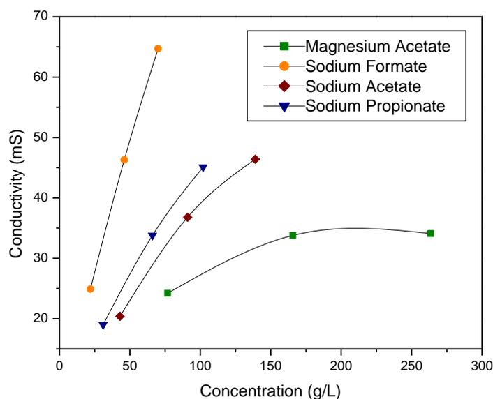
Figure 5. Conductivity-concentration relationship for each draw solution at concentrations corresponding to osmotic pressures of 1.4 MPa, 2.8 MPa, and 4.2 MPa.
