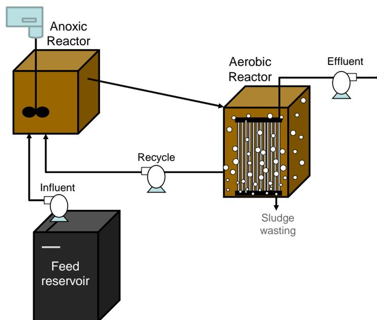
Figure 6. Schematic of laboratory-scale MBR system. Samples were collected from this system for batch experiments.
