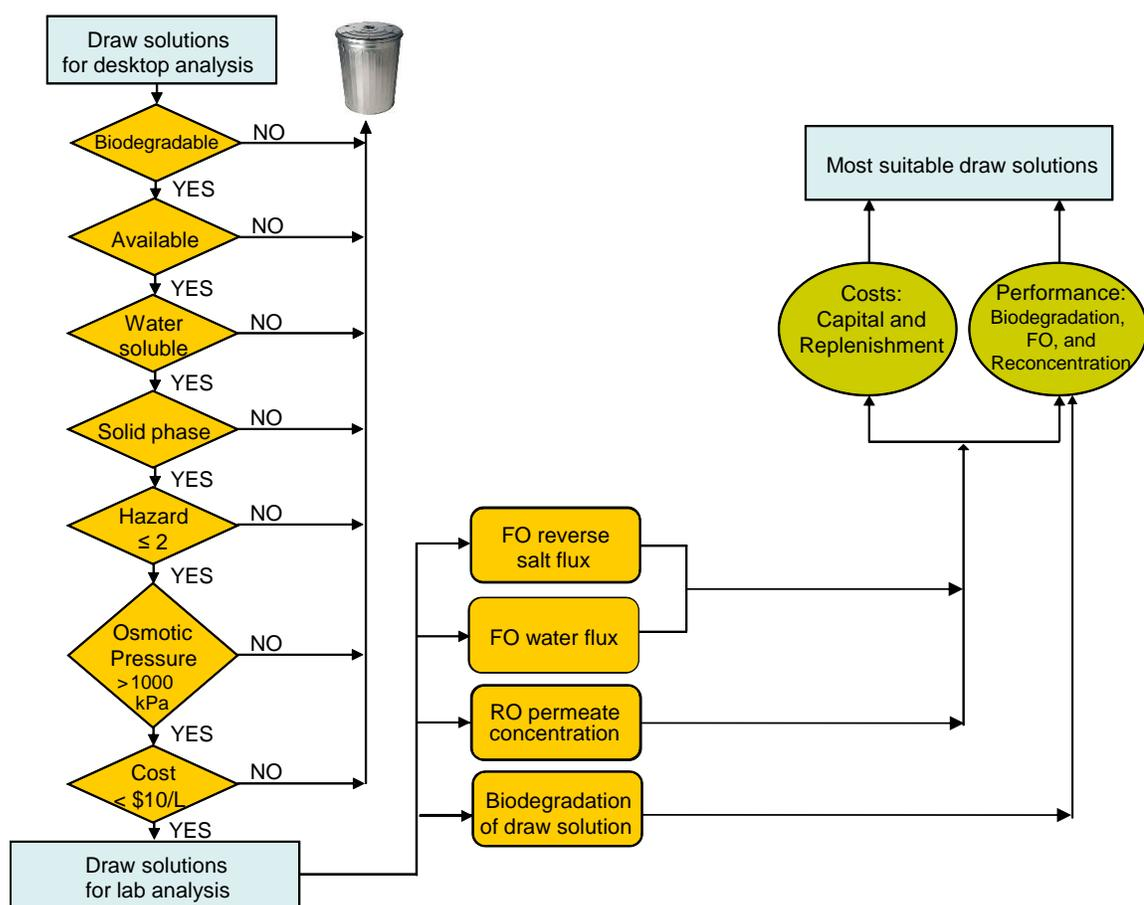
Figure 3. Flow diagram for draw solution selection for osmotic membrane bioreactor. Figure adapted from Ref. [5].
