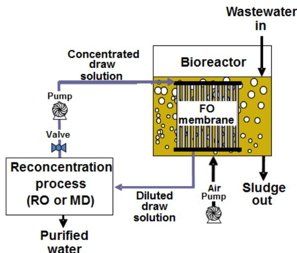
Figure 1. Schematic of an OMBR system. Figure adapted from Ref. [2].
