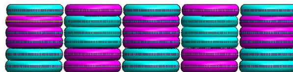
Figure 2: Ideal alignment of p type (blue) and n-type (pink) compounds in a bulk heterojunction cell.
