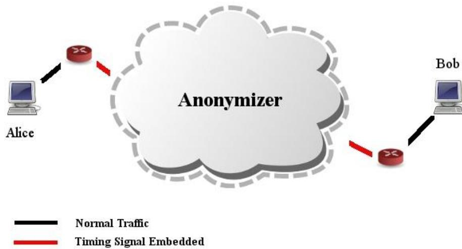
Figure 3.5: The timing signal is inserted and removed from the circuit.
