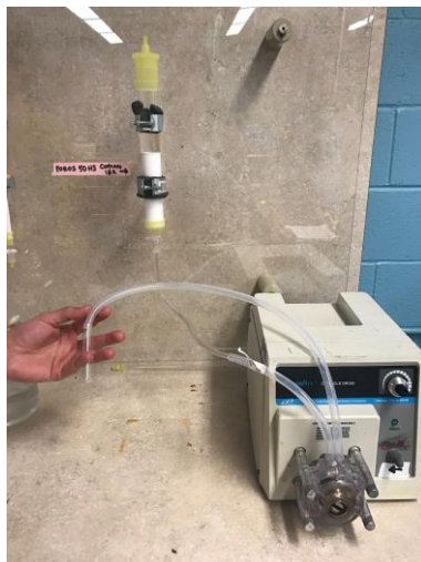
Figure 8: Cation chromatography column and pump setup.
