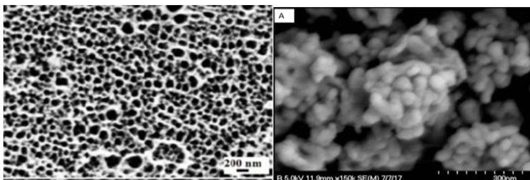
**Figure 3. SEM Image of Ta<sub>2</sub>O<sub>5</sub> and TaON.** The images above show the surface topography of tantalum pentoxide (left) (Minagar et. al. 2015) and tantalum oxynitride (right).
