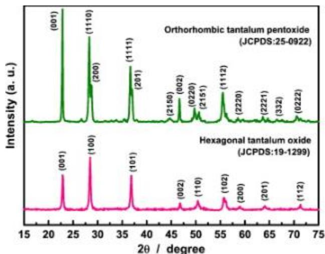
**Figure 2. XRD of Tantalum Pentoxide and Tantalum Oxynitride.** X-ray diffraction of  $Ta_2O_5$  powder (green) and TaON powder (pink) are displayed. The intensity, counts, indicates the unique crystalline structure of the two photocatalysts.
