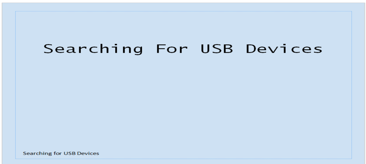
Fig. 17: This screen will display when the user selects the transfer rectangle at the menu screen. The goal is to add an indicator so the user isn't just looking at text when waiting for a device to be found.
