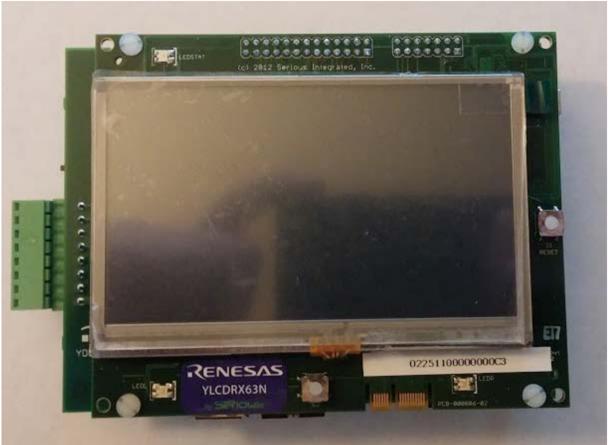
Fig. 26: This is the touch screen of the Renesas Embedded GUI and Communication Solution Kit. This is the main feature that the user will use to input and receive information.
