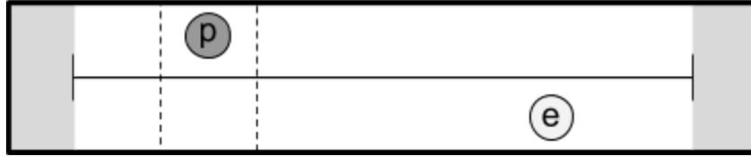
Figure 6: The fence escape game has two players, a pursuer  $p$  and evader  $e$ . The evader's goal is to get around the fence to the grey shaded  $X_{\text{goal}}$  without being within the dashed capture zone of the pursuer.
