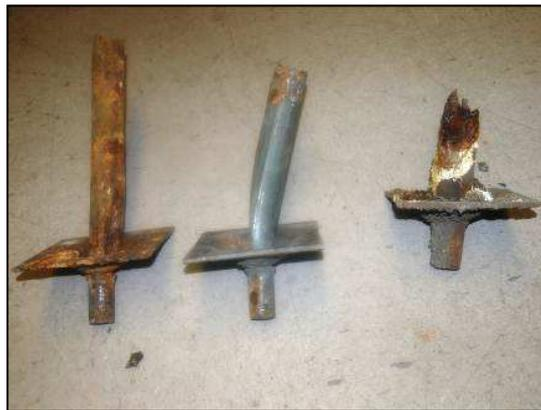
Figure 7: Bolts Failed due to Corrosion at Mine 2
