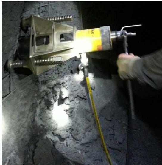
*Figure 5: Pull-Testing Equipment at Mine 2*
