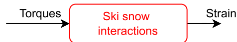
Figure 3.2: Simplified block diagram of ski snow system, showing a transfer function between the skier's inputs and the measurable strain output.
