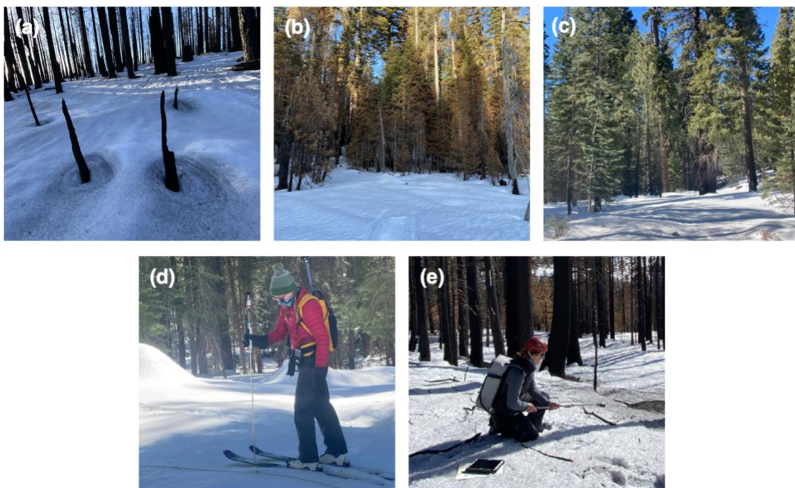
Figure 3. Photos from three field sites in the Creek Fire near Huntington Lake, Calif. (a) High burn severity, (b) moderate burn severity, and (c) unburned on 27 February 2021. (d) Snow depth measurements in an unburned forest using a MagnaProbe and (e) Albedo measurements in a high burn severity forest using the Spectral Evolution RS-3500 Portable Spectroradiometer™. Photo credits: Anne Nolin (a-d), Ben Hatchett (e).
