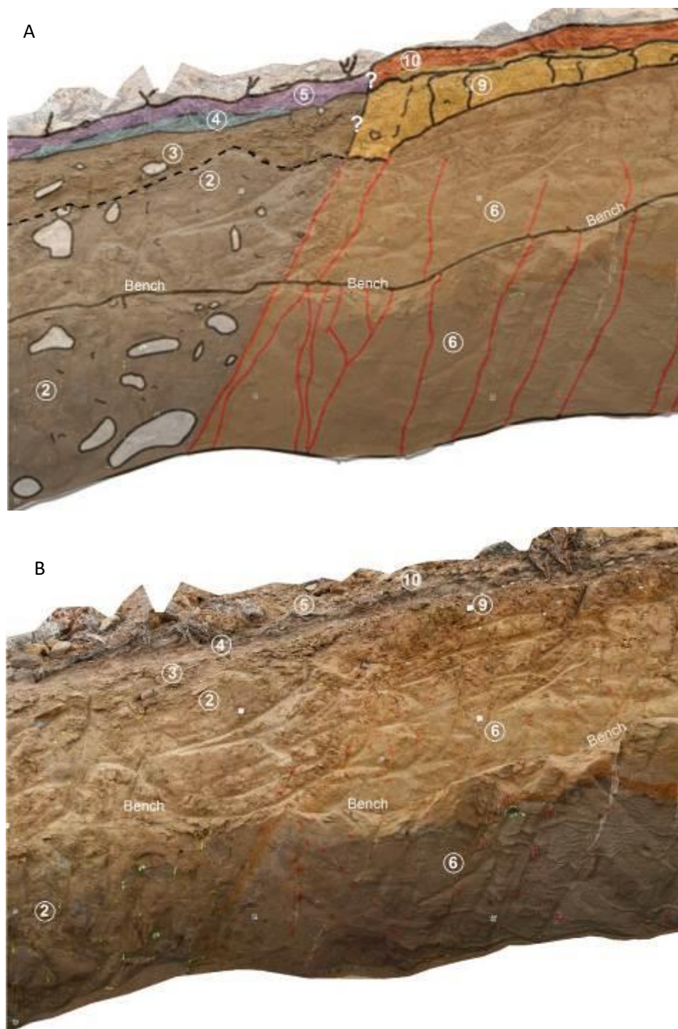
Figure B2. A) Enlarged trench photo orthomosaic of south wall with log mapping overlay at section of fault with unit labels. B) Enlarged trench photo orthomosaic of south wall with only labeled units.
