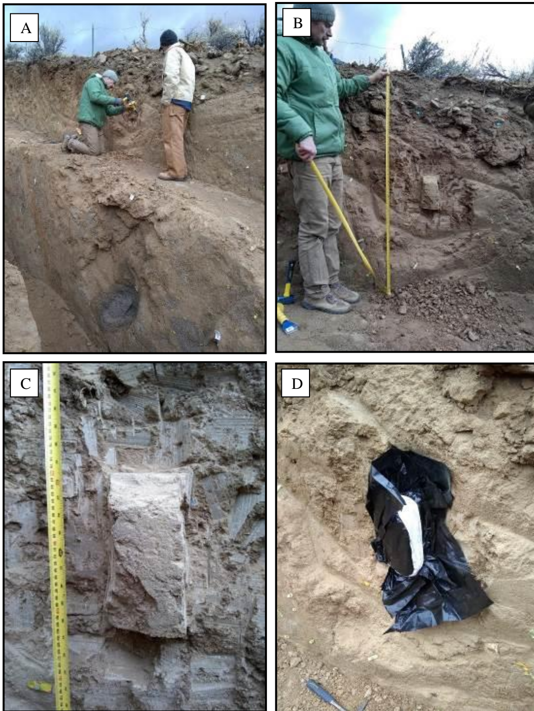
Figure C3. Photographs of OSL block sample collection. A) Using the electric hand saw to cut out block sample. B) Measuring height of collection to surface. C) Measuring size of block. D) Covering sample with 4 mil light proof plastic.
