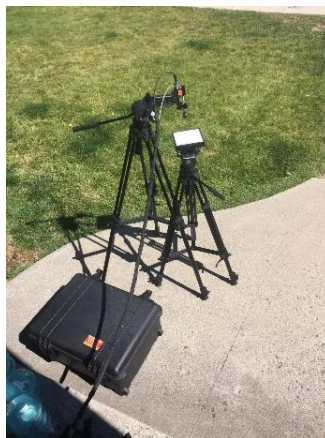
Figure 2. 6: Experimental setup for spectral reflectance factor measurements.
