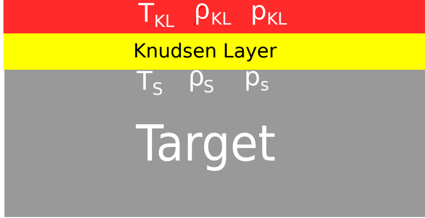
Figure 2.2 This sketch shows T_s , \rho_s , and p_s at the surface. The new parameters, T_{KL} , \rho_{KL} , and p_{KL} , represent the new equilibrium established after the collisional processes in the Knudsen layer.
