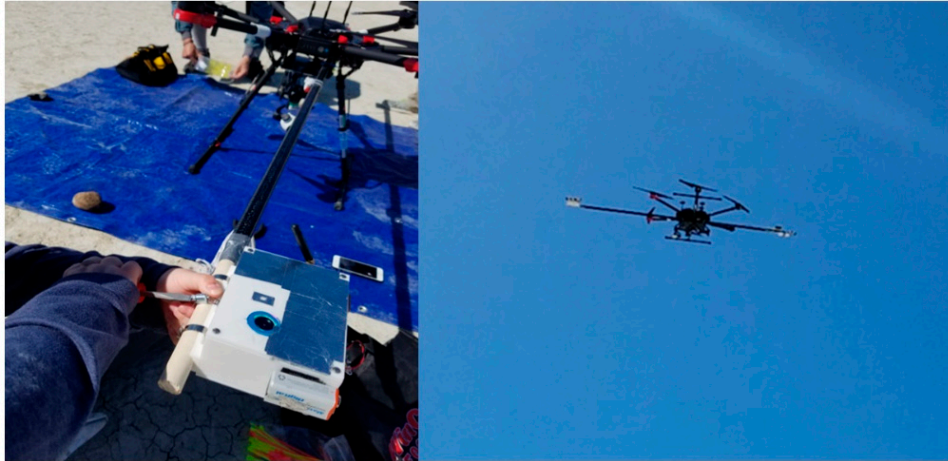
Figure 8. Configuration of instrument mounted to unmanned aircraft system (UAS). A long pole, approximately 2 m in length, was used to extend the instrument away from the body of the aircraft. This was done to limit the effects of the aircraft on albedo measurements, specifically those that would change the surrounding radiation field.
