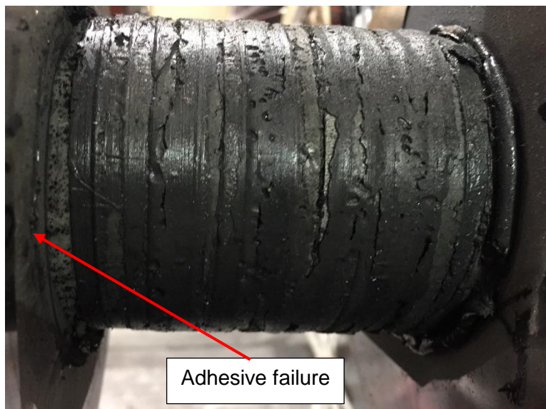
Figure 16. Failure of the MRE stacks of the bearing system.
