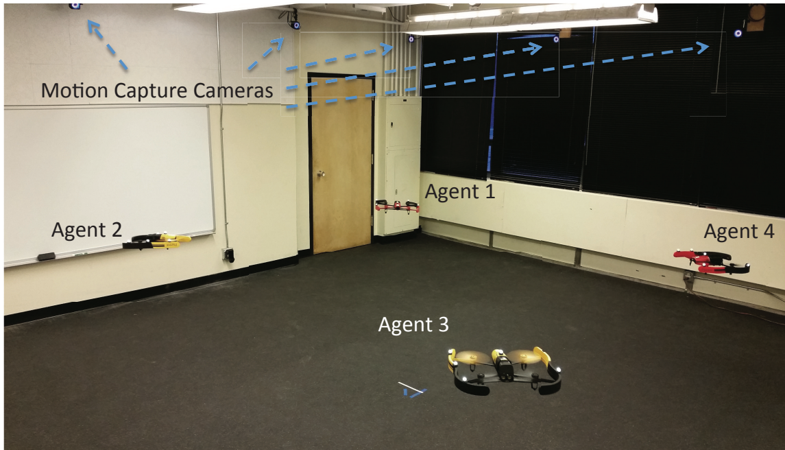
Figure 4.14: Experimental testbed: a set of four drones, a motion capture system, Ground Station computers, and WiFi links.
