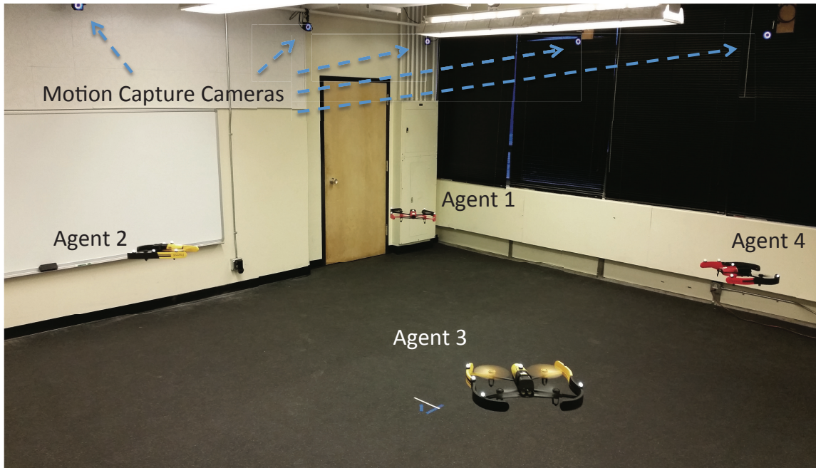
Figure 3.23: Experimental testbed: a set of four drones, a motion capture system, Ground Station computers, and WiFi links.
