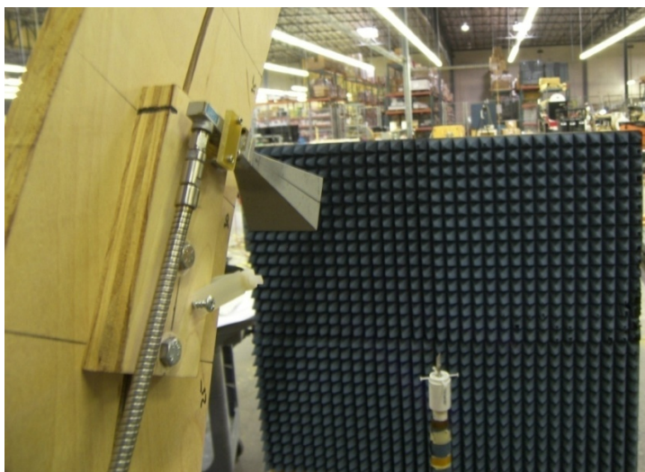
Figure 4-26. Source Antenna Mounted on the Wooden Arch at \theta = 60^\circ
