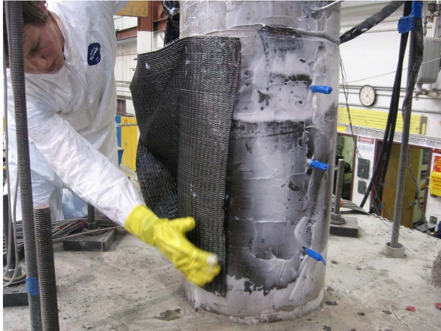
Fig. 2-54. FRP Wrapping for Column SC-2R
