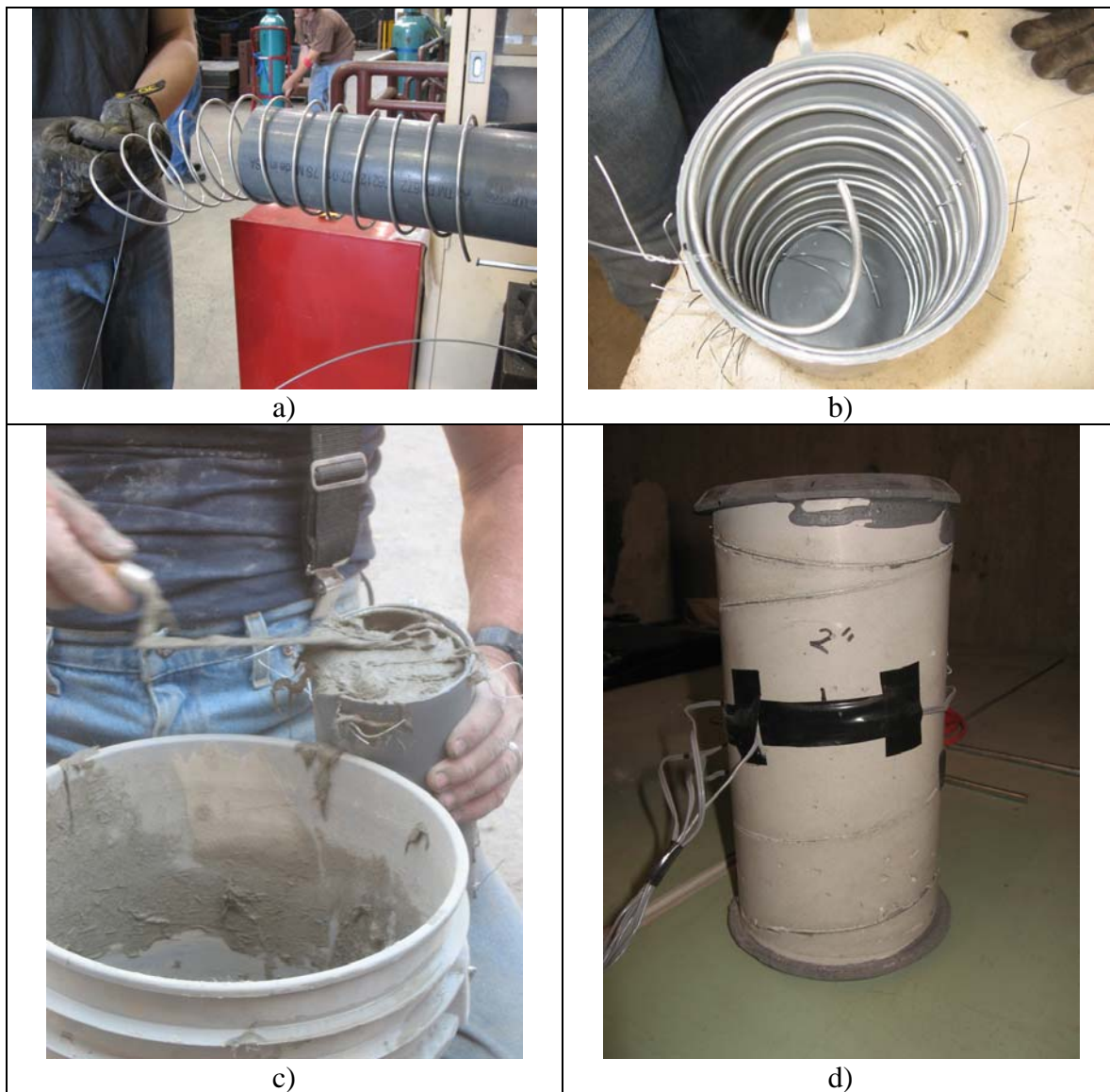
Fig. 5-6. Building the Test Samples Steps a) Rolling the Spirals, b) Adjusting the Spacing, c) Filling with ECC, d) Instrumentation
