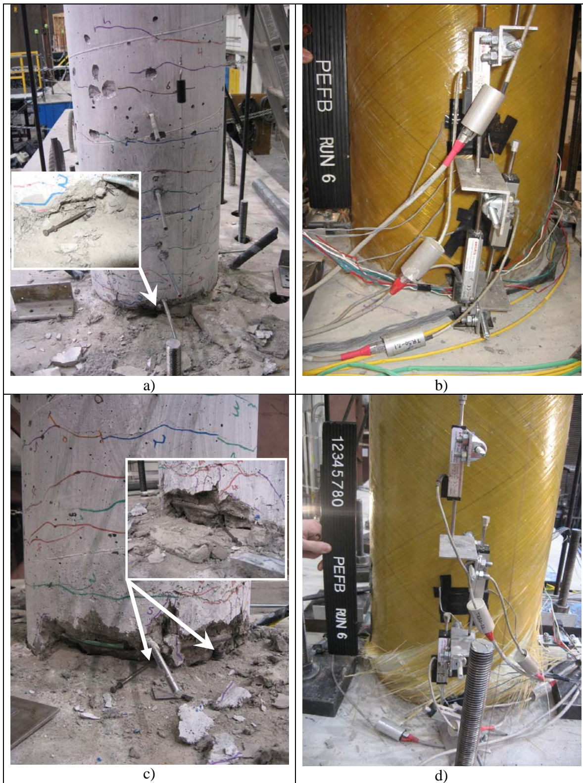
Fig. 4-12. Apparent Damage at 10% Drift for a) RC-ECC, North, b) FRP, North, c) RC-ECC, South, d) FRP, South
