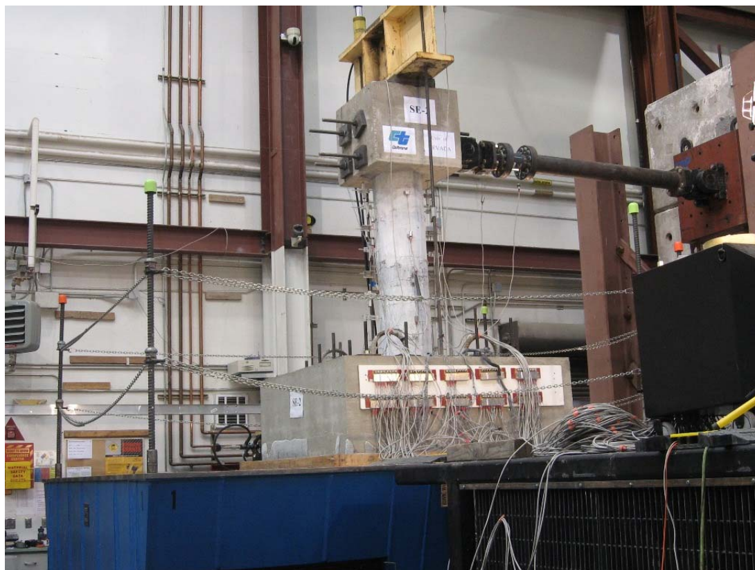
Fig. 2-48. SE-2 after Construction and Assembly
