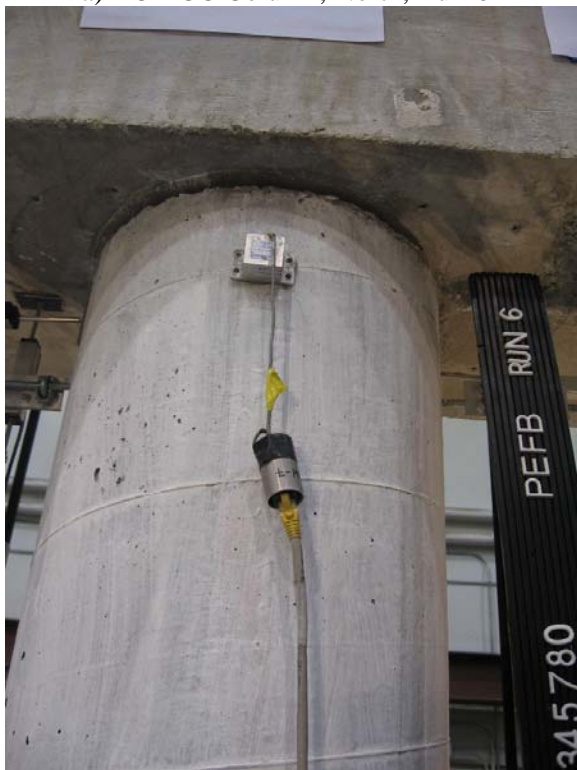
c) RC-ECC Column, East, Run-6
