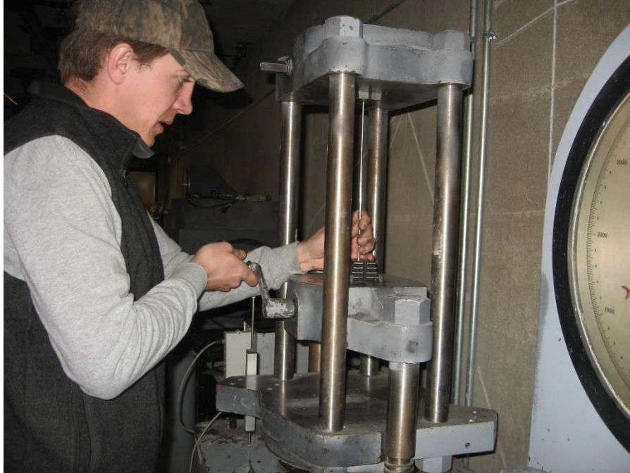
Fig. 5-5. Testing the Transverse Wires in Tinus Olson Testing Machine
