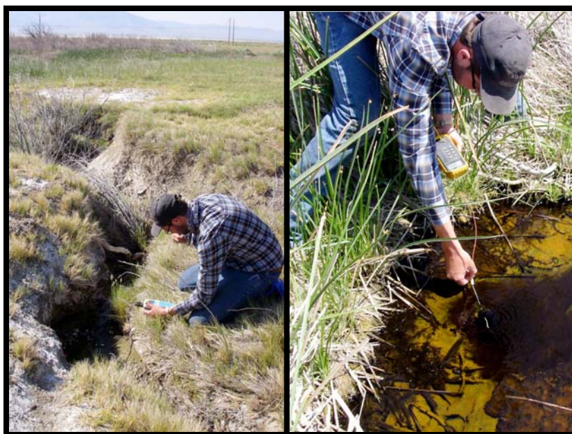
Figure 2.5. Pictures from the spring fluid survey. Field assistant C. Dudley measures pH/TDS (left panel) and temperature (right panel). Note that measurements are being performed where the fluid first comes to the surface.
