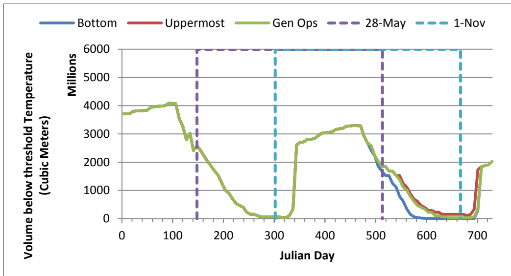
Figure 49. In-reservoir cold pool volume, calculated weekly for the two year drought, at or below the cold pool temperature threshold of 12.8°C for each TCD Schedule (bottom, uppermost and generalized operations). “28-May” and “1-Nov” refer to their corresponding calendar dates.
