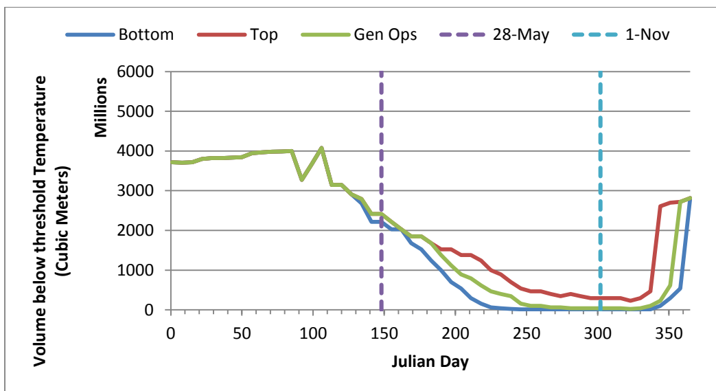
Figure 50. In-reservoir cold pool volume for the extreme dry year with low emissions air temperature increases, calculated weekly, at or below the cold pool temperature threshold of 12.8°C for each TCD Schedule (bottom, uppermost and generalized operations). “28-May” and “1-Nov” refer to their corresponding calendar dates.
