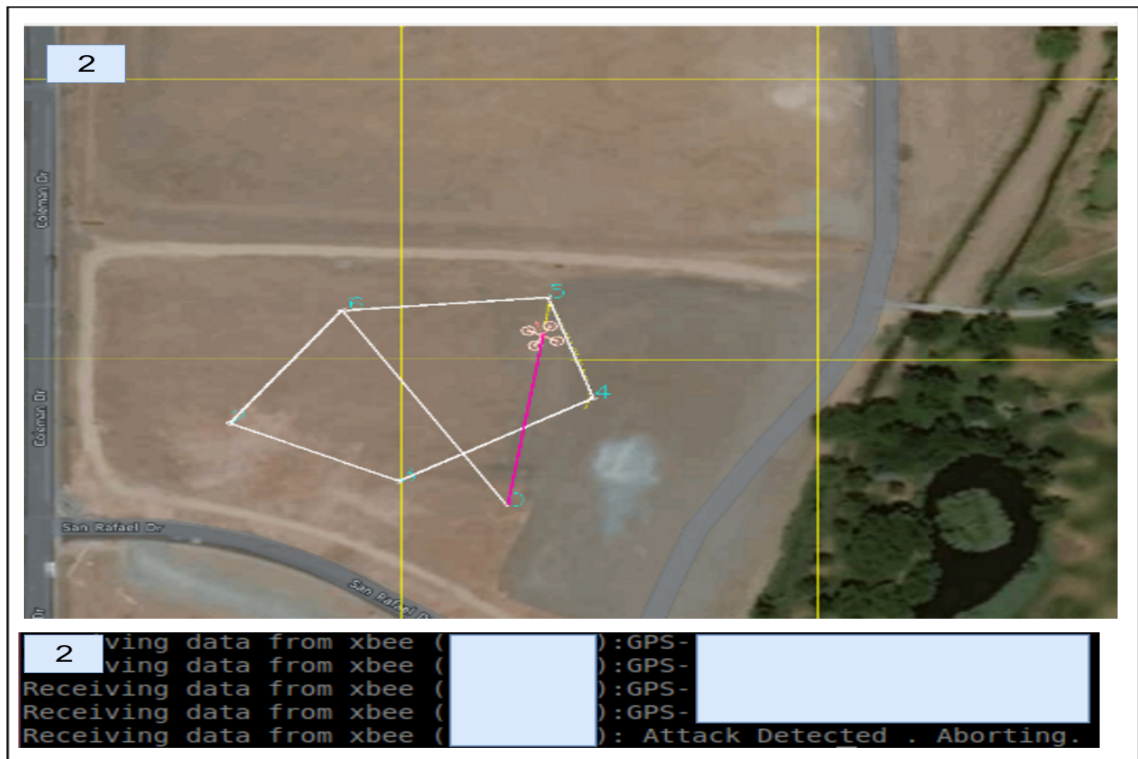
Figure 5.3: Waypoints set for the experiment in the second configuration. The attack was discovered after the UAV navigated from waypoint 5 and Return-to-Launch (RTL) was enabled.
