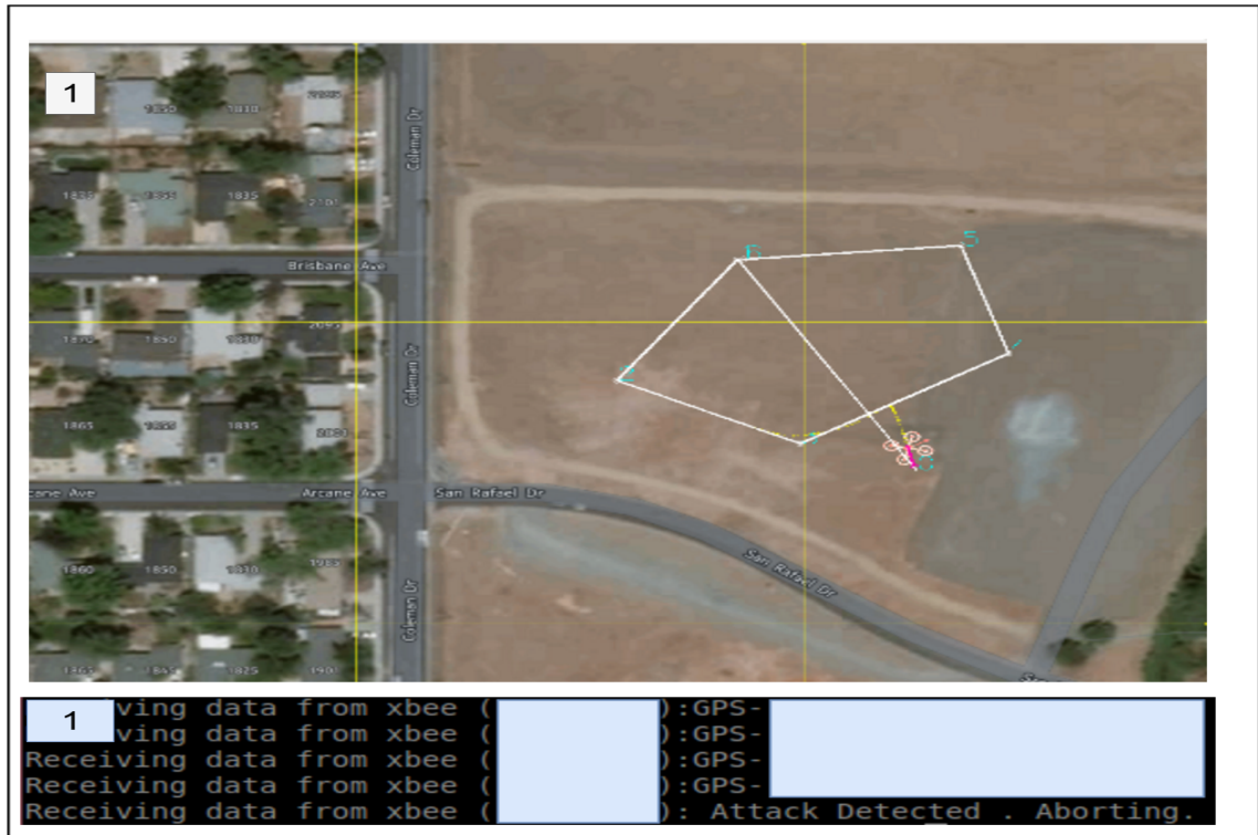
Figure 5.2: Waypoints set for the experiment in the first configuration. The attack was discovered after the UAV navigated from waypoint 3 and Return-to-Launch (RTL) was enabled.
