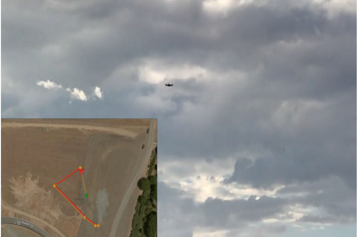
Figure 5.6: Waypoints set for the experiment in real time. The attack was discovered after the UAV navigated after waypoint 4 and Return-to-Launch (RTL) was enabled.
