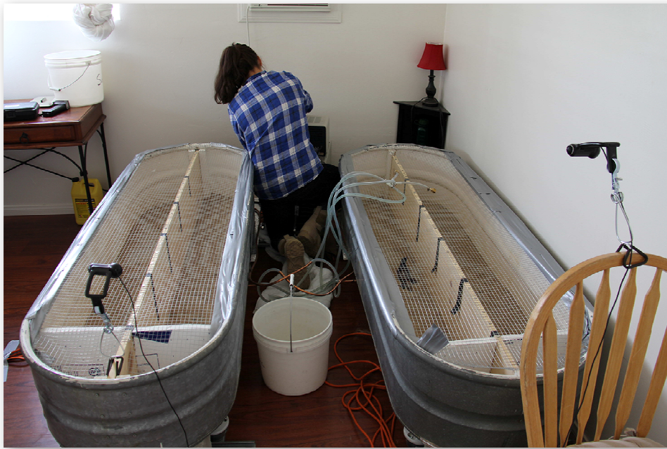
Figure 1: Two laboratory-controlled temperature gradients separated by a wood median equipped with thermal data loggers.
