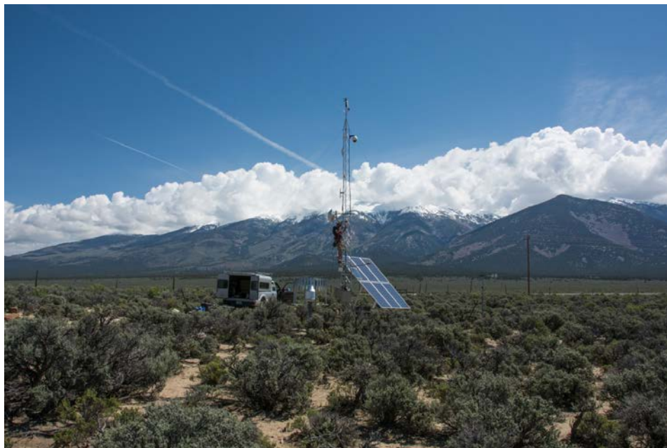
3.1.1: The author performs maintenance on the Snake Range Sagebrush observation station in Spring Valley in 2015. This site differs from the others in the study in the sense that it is not located within the mountain block and therefore is subject to different temperature, wind, and precipitation processes.
