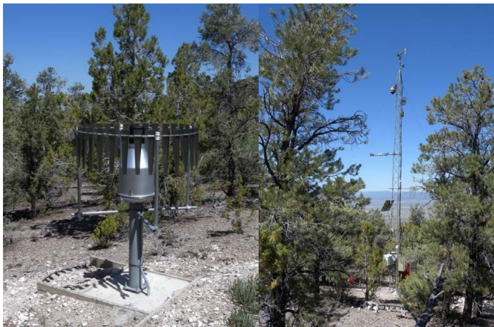
3.1.2: The Snake Range Pinyon-Juniper site is located in a relatively young woodland of moderate density and low canopy height (< 8 m). The meteorological tower (left) and Geonor precipitation gage (right) are sited in small clearings.
