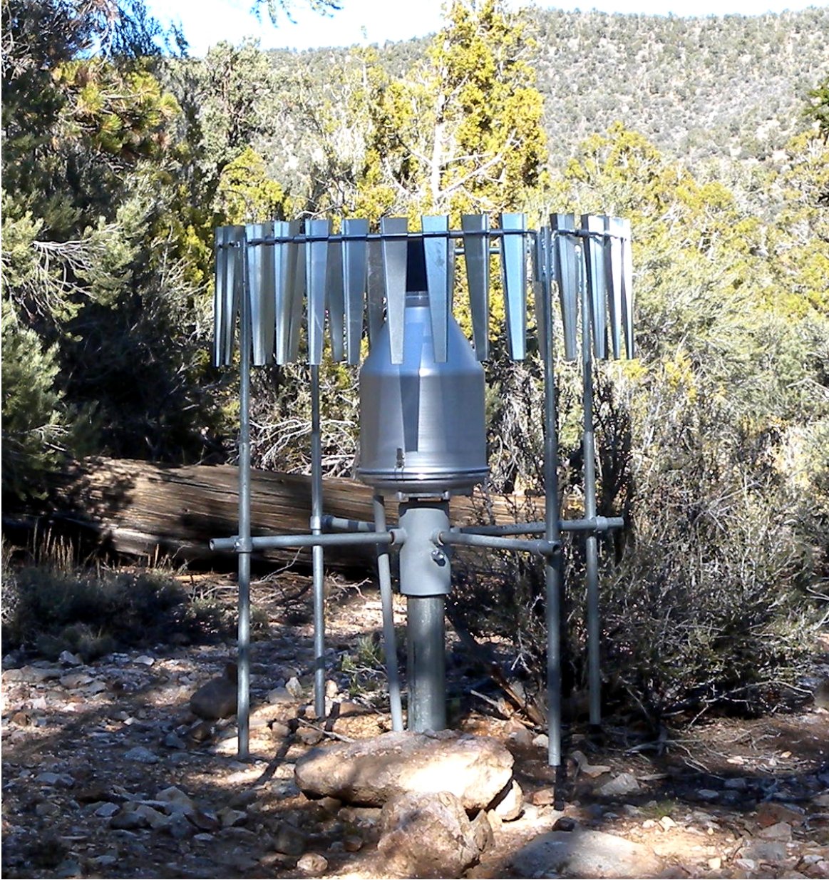
Figure 22. The Geonor T-200B precipitation mass weighing sensor.
