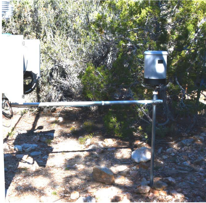
Figure 23. The Hydrological Services TB4 tipping bucket rain gage.
