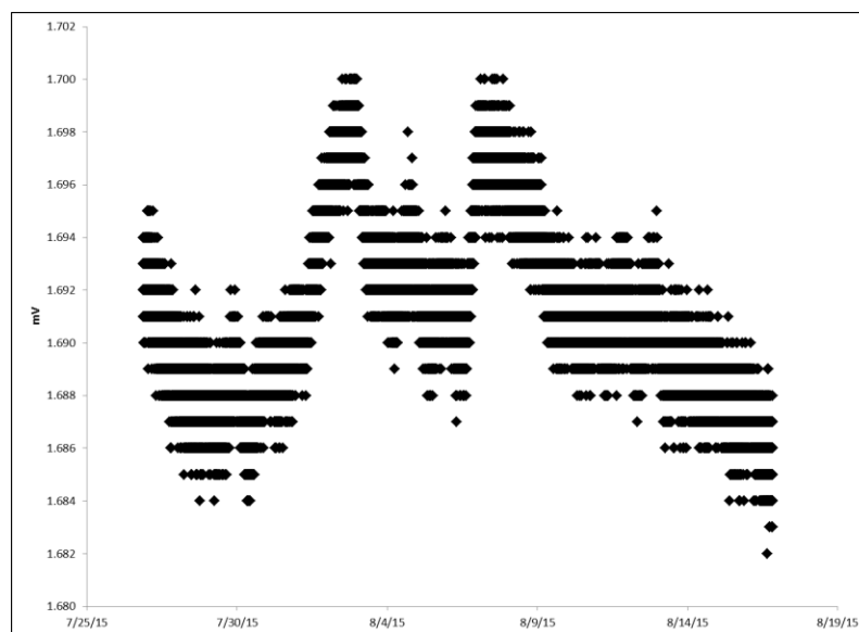
Figure 16. SWE sensor measurement fluctuates over the time period, due to electrical circuitry. The total change in measurement was equal to \pm 0.003 cm over this time period.
