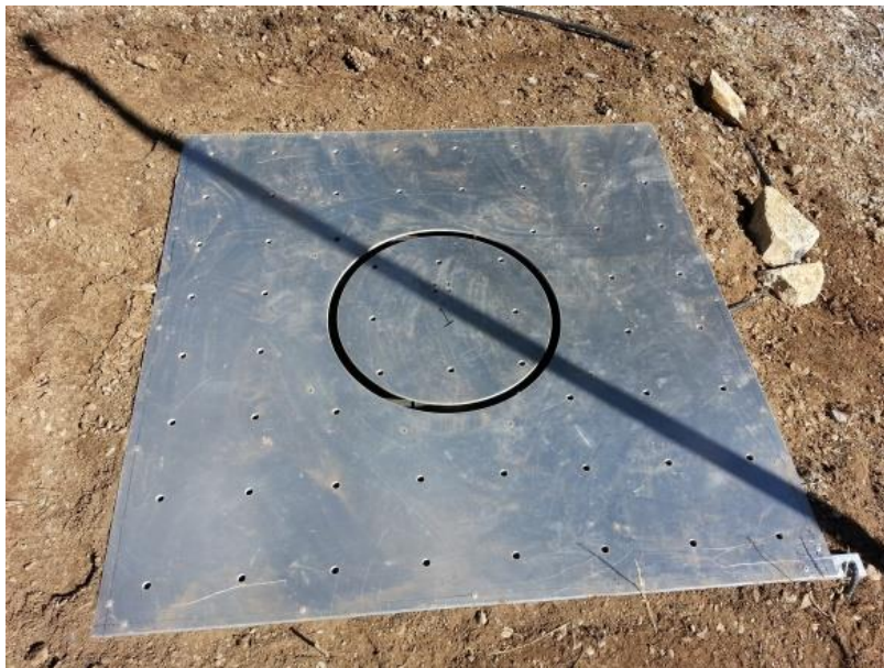
Figure 5. SWE sensor at the sub-alpine west site in the Snake Range, NV.
