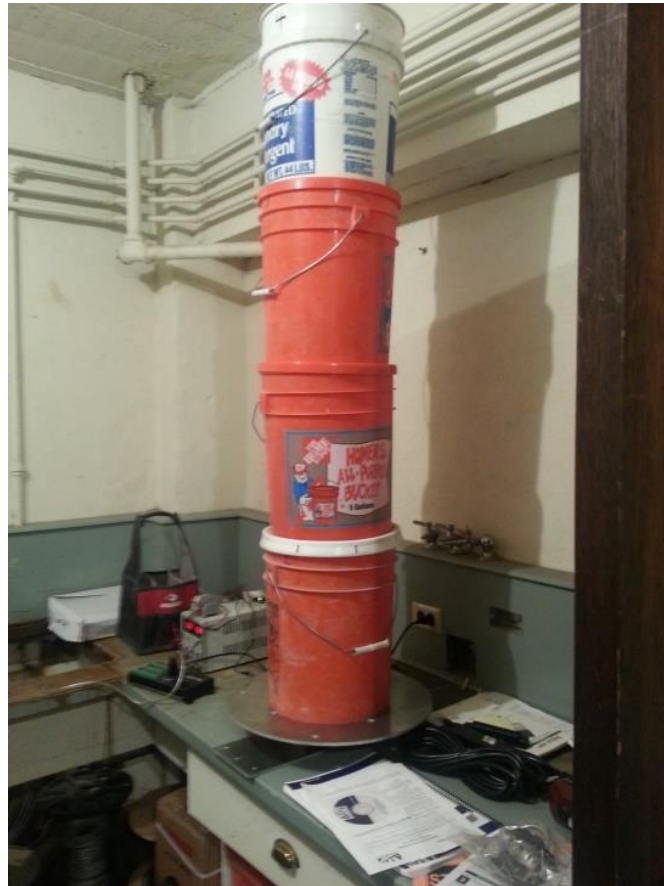
Figure 6. Calibration of weigh sensors using water and five gallon buckets.
