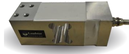
Figure 4. Loadstar RAP3 single point resistive load cell.
