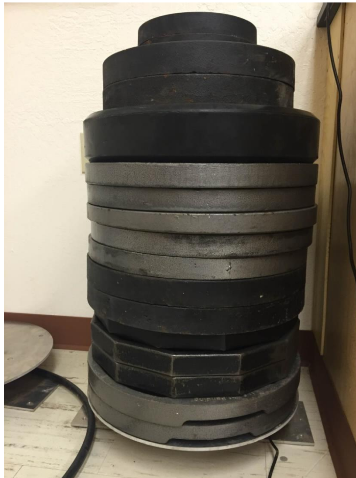
Figure 15. Laboratory test with a load of 306 kg, equivalent to 184 cm of SWE.
