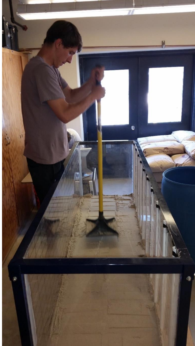
Figure 3-9: Preparation of Non-Liquefiable Layer
