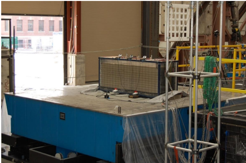
Figure 4-21: Test #53 Positioned on Biaxial Shaking Table
