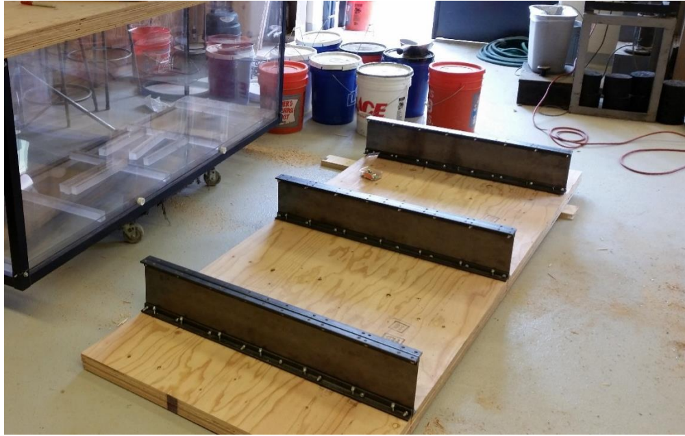
Figure 3-3: Fabrication of Shake Table
