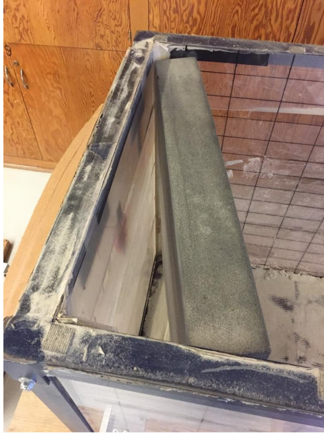
Figure 4-5: High Density Foam for Boundary Effect Reduction
