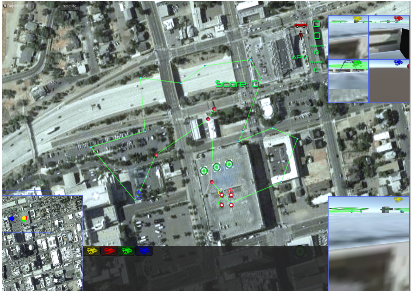
FIGURE 5.10: Figure showing the shortest path found by the GA for 18 waypoints. Smaller Aqua points are the waypoints the UAV has to visit. Bigger red points have been already visited by the UAV.
