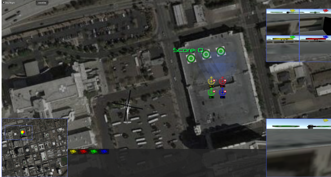
FIGURE 5.4: RenoRescueSim user interface. Center: is the main view, where a user can get a top-down view of the world (rendered from Google Maps tiles); Bottom-Left: minimap view of the entire city, with area viewable in the center panel shown (blue-box); Bottom-Right: View from currently-selected UAV's camera; Top-Right: Views from all UAV's cameras
