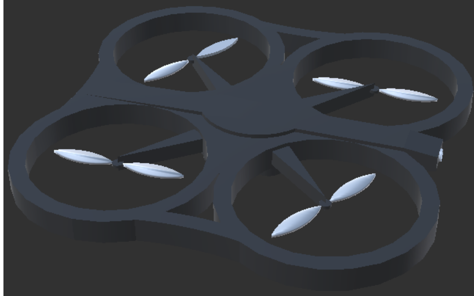
FIGURE 5.1: UAV model used in the simulator. This UAV has two cameras. One for looking directly in front and other for looking below. It also simulates all the sensors and actuators the hummingbird robot has (e.g., GPS, wireless communication, and inertial guidance system).
