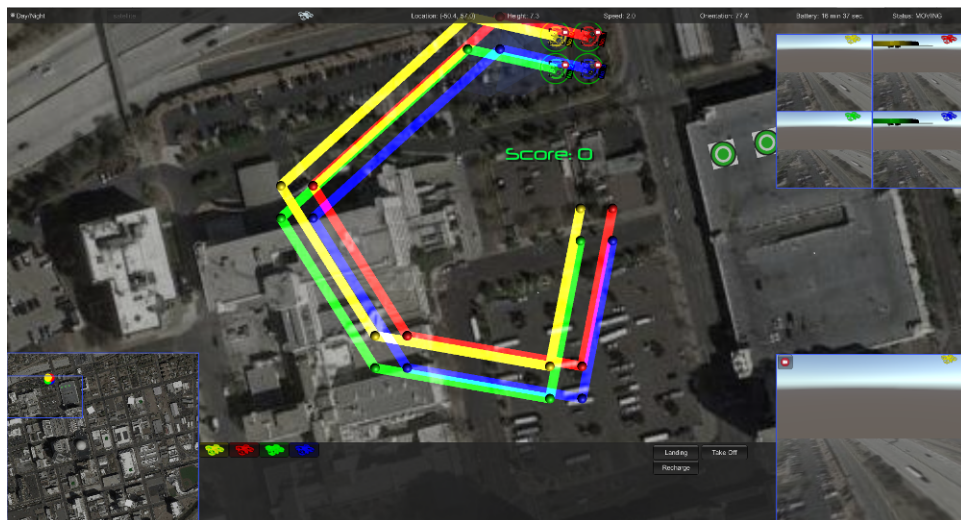
FIGURE 5.7: Multiple-UAV navigation with several waypoints set for multiple UAVs to move in formation (Red, Yellow, Cyan, Blue lines) (Level 3 autonomy). Waypoints can be set by selecting multiple UAVs and right-clicking either in the center panel or in the minimap view.
