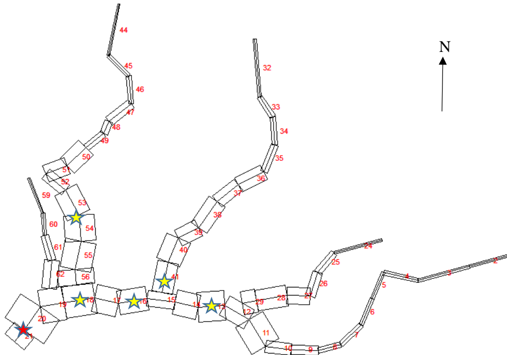
Figure 12. Spatial location of CE-QUAL-W2 model segments for Shasta Reservoir. Model segments corresponding to temperature profiles taken in 1995 and used for calibration are noted with yellow stars. The general location of the DTS vertical profile and sonde data profiles is indicated with a red star.
