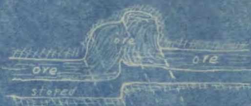
'right angle fault zone' - ore in hanging wall.
