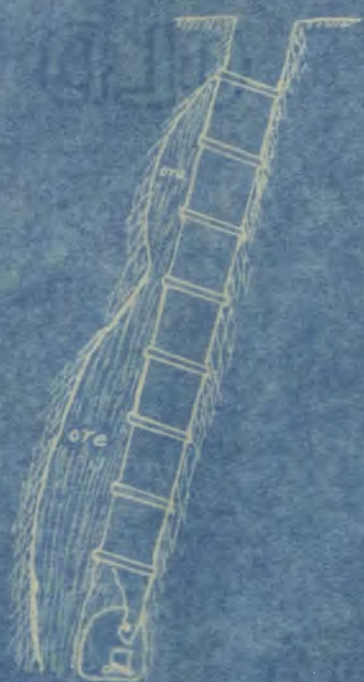
Cross section - ore bounded by fault slips on the hanging wall.
