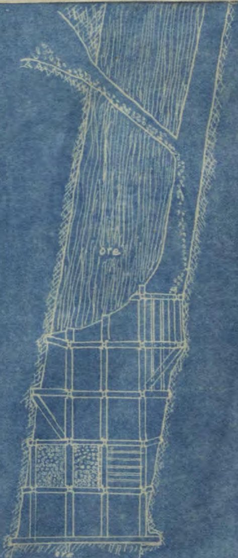
Cross section waste raise in hanging wall
