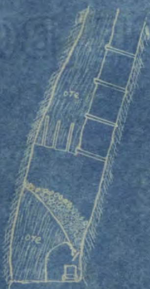
Cross section of 'shrinkage' stope.
