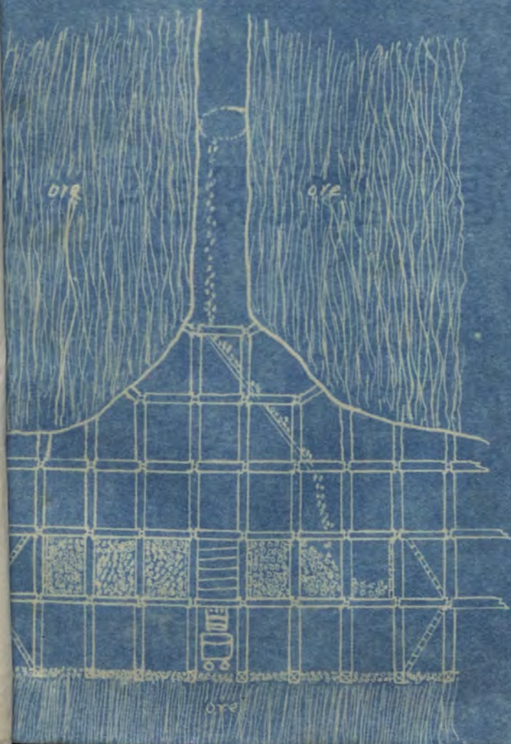
Longitudinal Section square sets filled with waste
