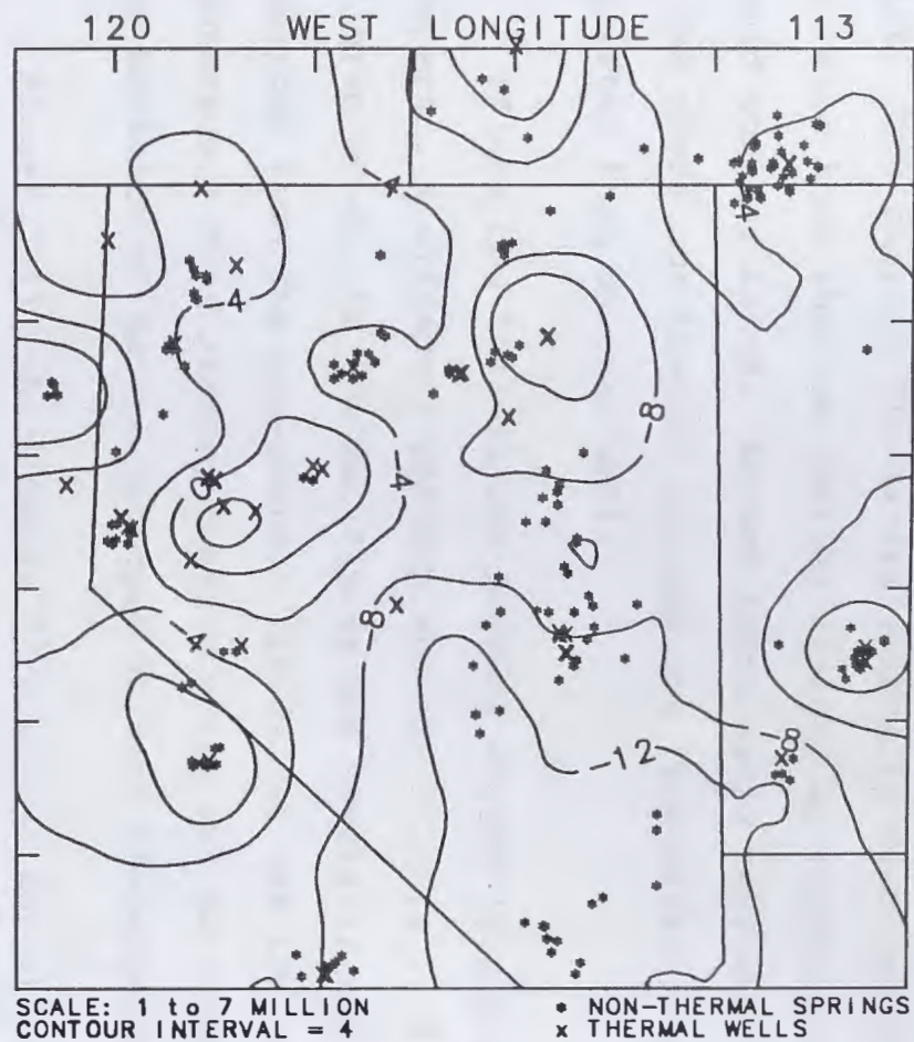
Figure 7.14: Deuterium permil difference for thermal well minus non-thermal springs. The thermal wells are also more isotopically depleted than the non-thermal springs, as indicated by the negative (solid) contour lines.
