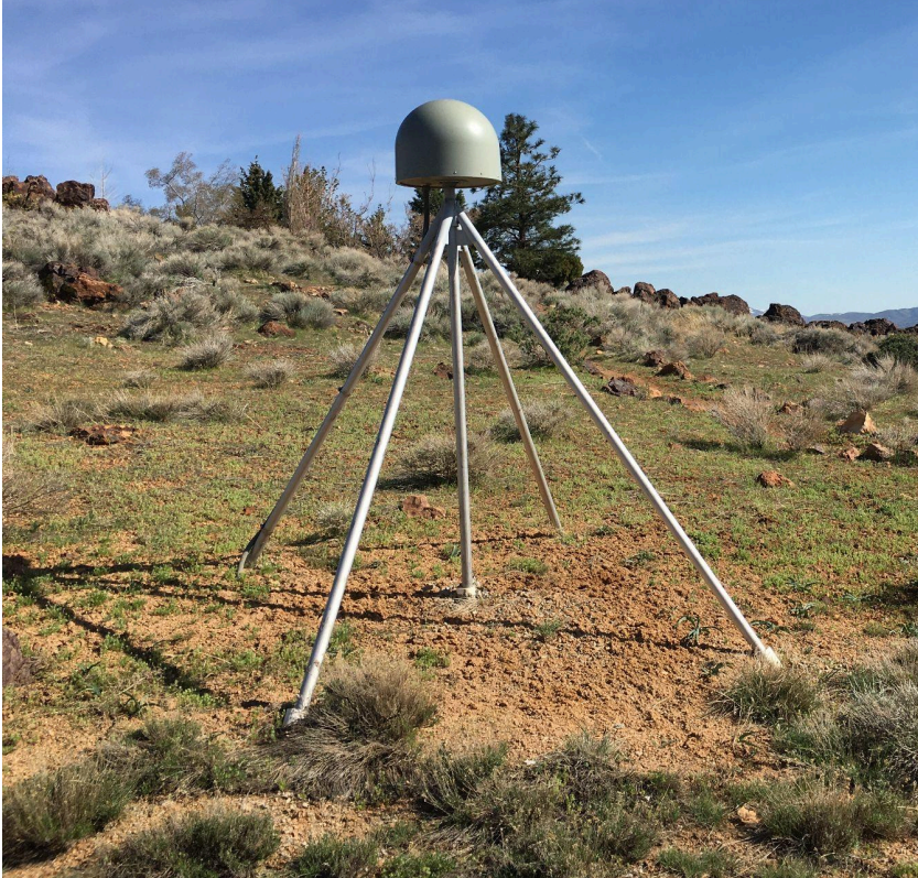
Figure 1.3: An example of a deep-drilled braced monument, station P090 located in Reno, NV.
