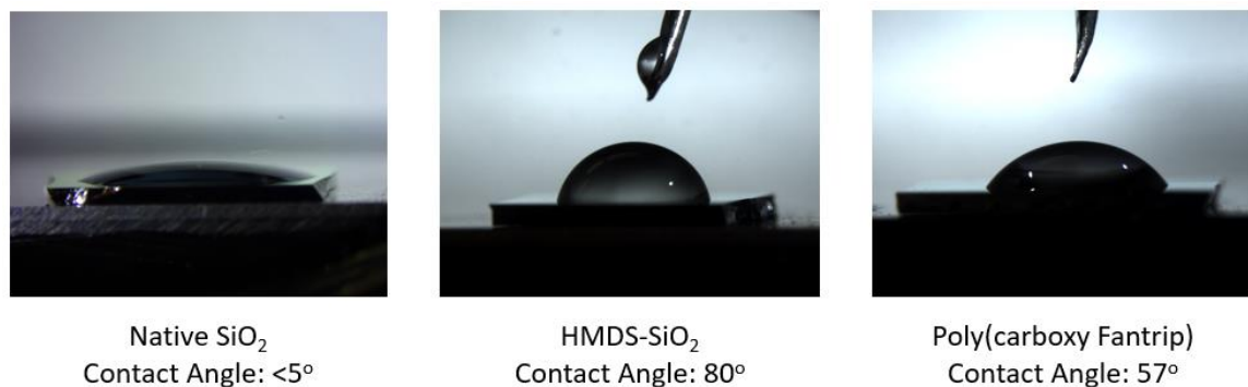
Figure 3.29 Contact angle of different substrates: Measuring the differences in contact angle of different surfaces offer insight to a change in surface chemistry.
