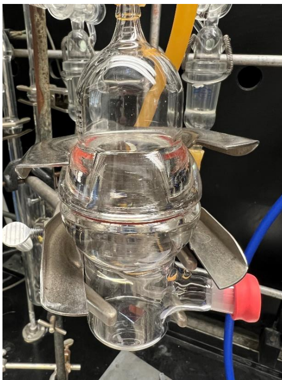
Figure 3.27 Experimental setup of vacuum chamber used to functionalize poly(carboxy fantrip) surface: Custom made vacuum chamber with HMDS-SiO 2 chip harboring deposited film on bottom.
