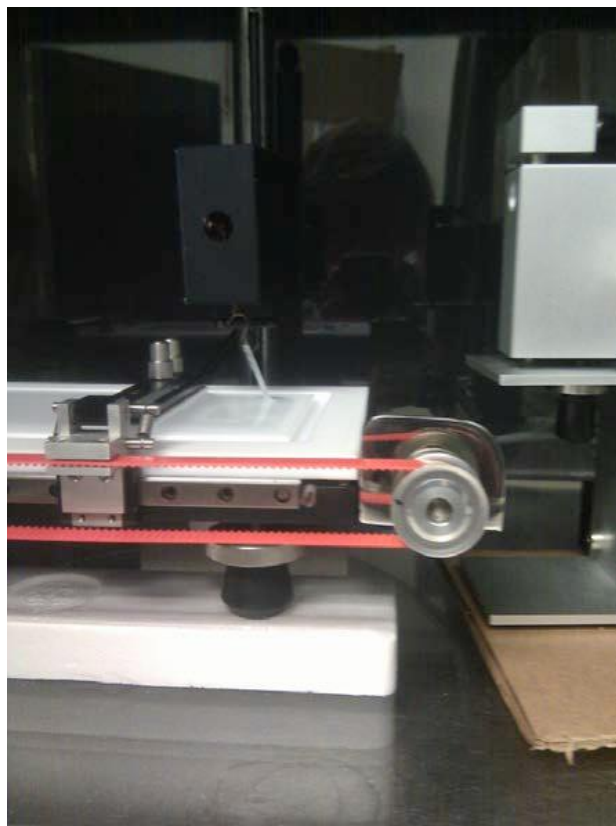
Figure 3.5 Single Barrier Trough: Image depicting large deflection of the Wilhelmy plate during compression of antrip-DEG. Upon relaxation of barrier, Wilhelmy plate falls back to a vertical position. Image taken by Daniel Murray.
