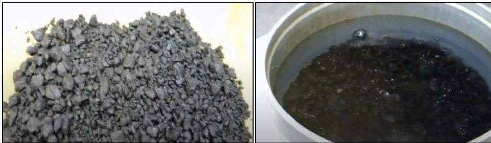
Figure 14. Loose Mixture for Gmm (left), Loose Mixture in Vacuum machine.
