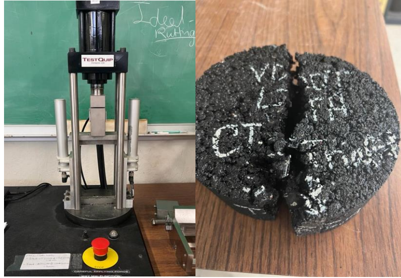
Figure 15. IDT-CT machine (left), IDT-CT tested sample (right)
