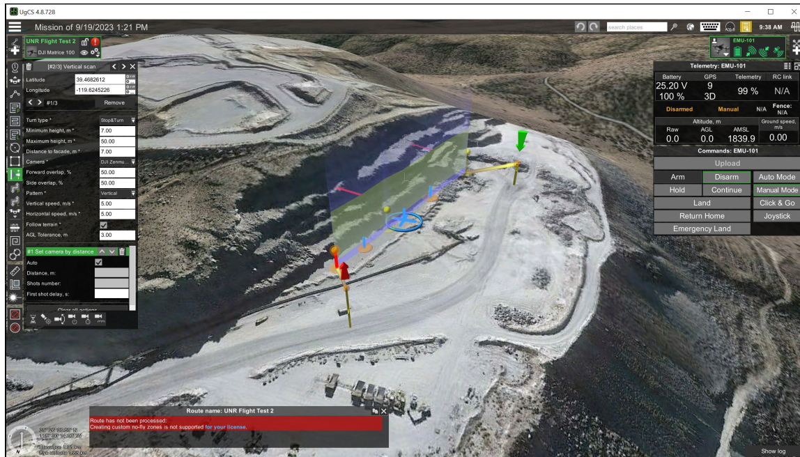
Figure 13 User interface of UgCS drone application. The green rectangle is the parameter of the drone flight path.
